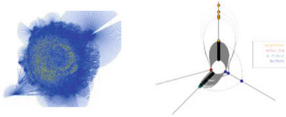
Fig. 9 Example of conventional “hairball” force graph (left) of cyberattack data and an example of the same data visualized as a four-axis hive plot mapping (right) (shown for topologic comparison only)
