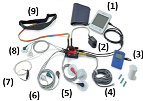
Fig. 2. The various medical sensors that can be used in this platform all connected to the e-health sensors shield. The figure depicts the following sensors: (1) Blood pressure sensor, (2) Oxygen in blood sensor, (3) Glucometer sensor, (4) Body temperature sensor, (5) Electrocardiogram sensor, (6) Electromyography sensor, (7) Airflow sensor, (8) Galvanic skin response sensor, (9) Patient position sensor [19].
