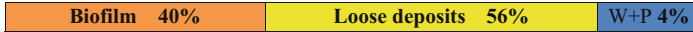
Fig. 9.1 Comparison of viable biomass in percentage (%) (as inferred from ATP results) of different phases within 1 m-long water pipes (PVC, 110 mm in diameter): from left to right pipe wall biofilm, loose deposits, and water + particles (W+P) (adapted from Liu et al. 2014a)
