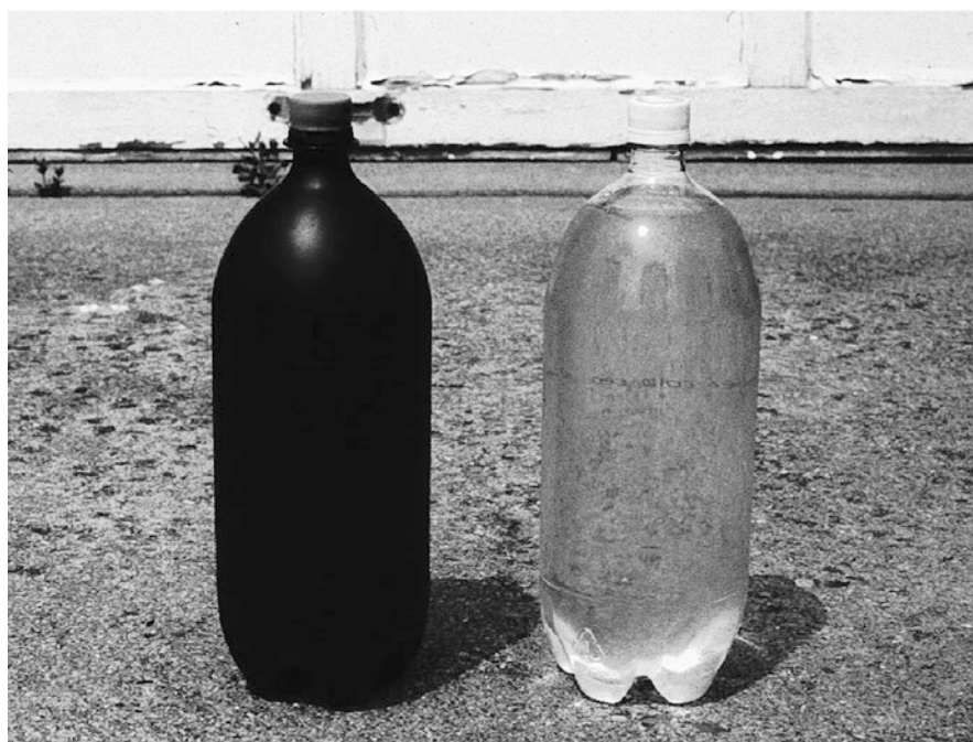
Fig. 8.35 Solar pasteurization of water also is called solar disinfection and abbreviated SODIS. The upper image is titled “Indonesia-sodis-gross” by SODIS Eawag and is being used under the Creative Commons Attribution 3.0 Generic license. The lower image shows water in a clear plastic
