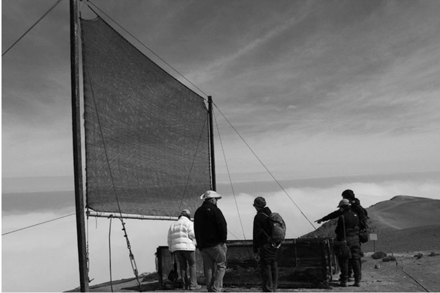
Fig. 8.12 This image shows a fog harvesting net above a water collection trough. The water which condenses on fog nets drains into the collection troughs which are mounted beneath those nets. That collected water then drains into either a storage tank or a piping system by which the water is distributed to a community. The image is titled “Atrapanieblas en Alto Patache” by Pontificia Universidad Católica de Chile and used under the Creative Commons Attribution 2.0 Generic license
