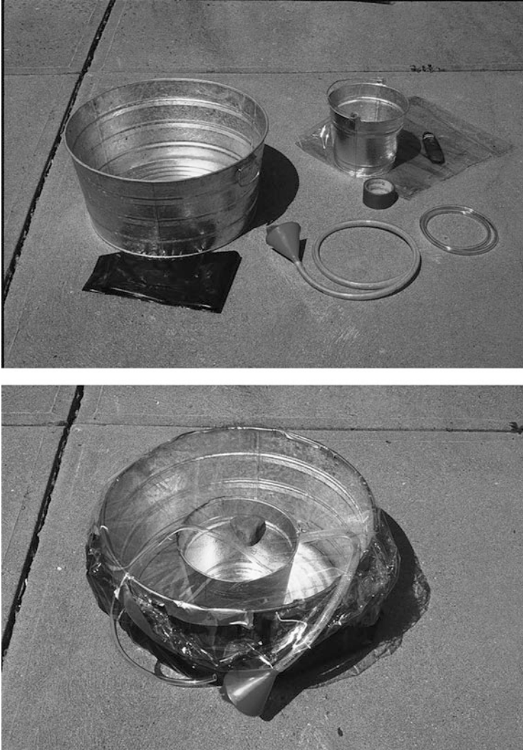
Fig. 8.37 These images show the components and assembly of a solar still designed for using heat from sunlight to distill water. Usage of these images is courtesy of the author
