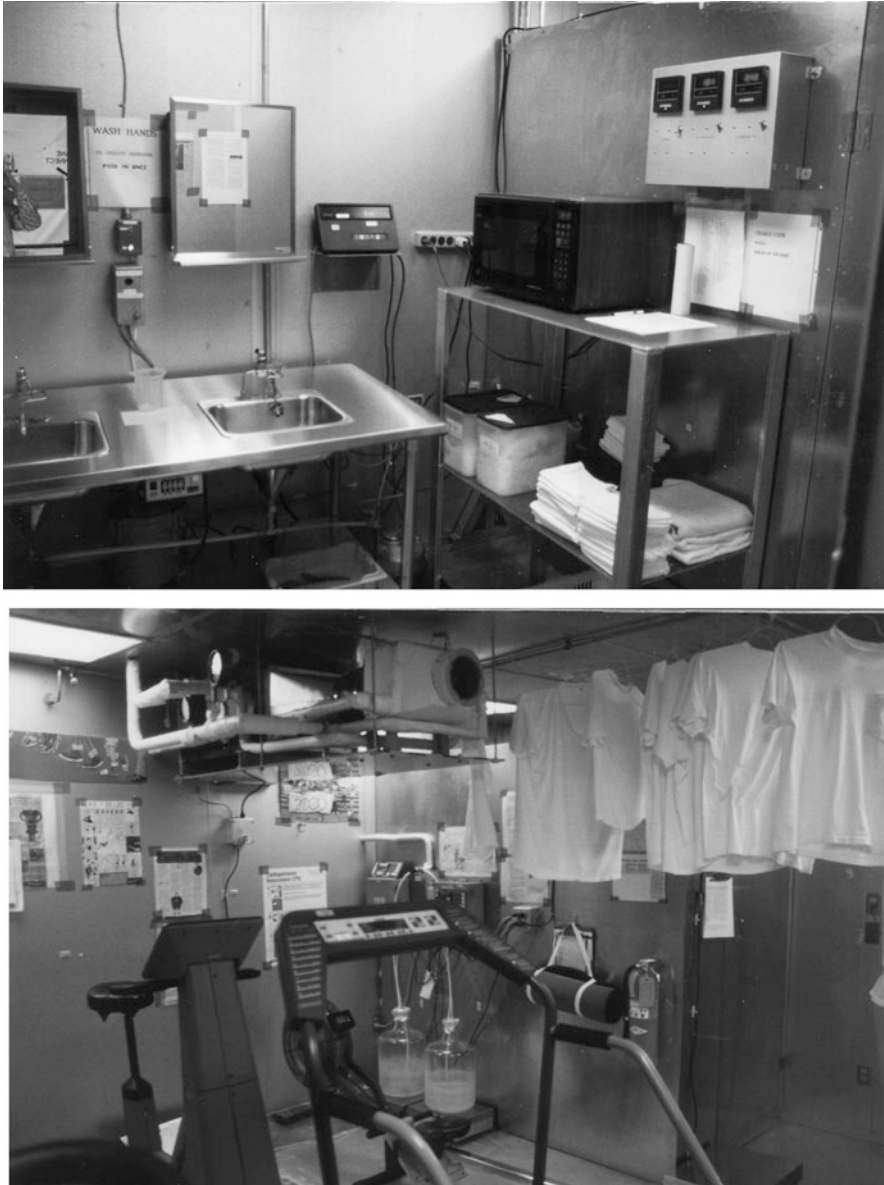
Fig. 8.40 These images show additional sources of water that were used for evaluating the water reclamation unit developed at NASA in Huntsville, Alabama for the International Space Station. The upper image shows a sink used for hand washing and dental hygiene plus a microwave oven for heating meals. The lower image shows exercise equipment and t-shirts hung to dry. In the bottom center area of the lower photograph condensate from a room dehumidifier can be seen collecting into glass storage containers. Usage of these images is courtesy of the author
