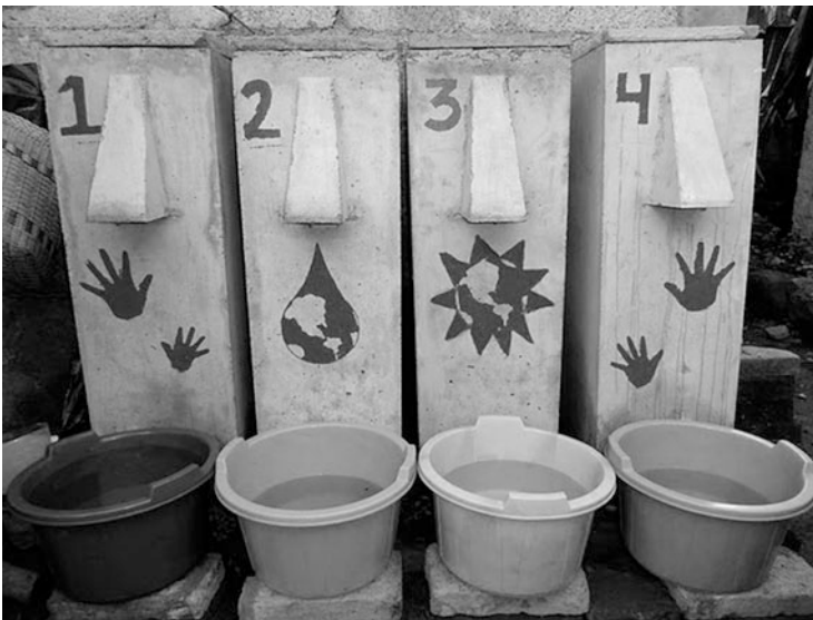
Fig. 8.29 This image shows biosand filters, they are small volume slow sand filters used to provide water for drinking and washing. The image is titled “Biosand Filters in Guatemala” by Nora. jeanine530 and used under the Creative Commons Attribution 3.0 Generic license
