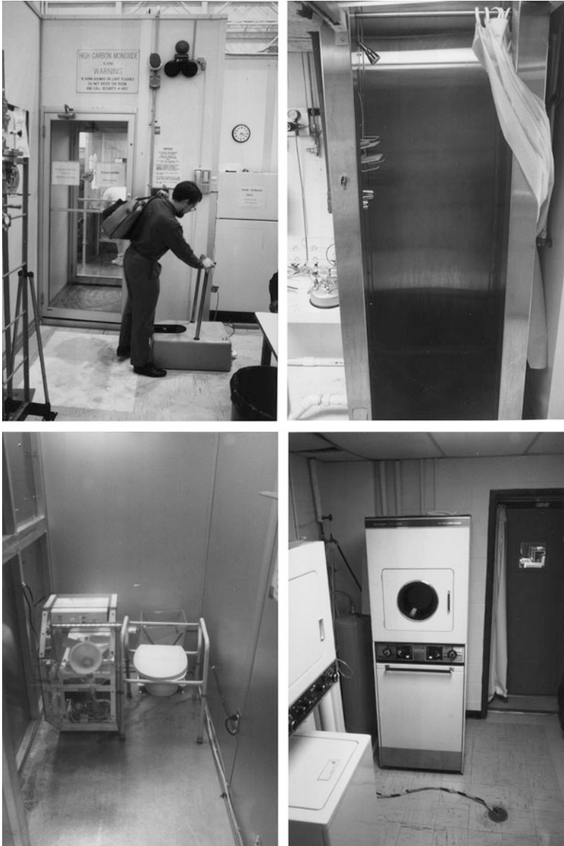
Fig. 8.39 These images show sources of water that were used for evaluating the water reclamation unit developed at NASA in Huntsville, Alabama for the International Space Station. Most of the water was collected from sources located within in a small temporary structure contained inside of a much larger building. Clockwise from the upper left these photographs show: a person using a powered shoe brush to clean their shoes before entering the temporary structure; a shower bath; a laundering machine and clothes dryer; and a toilet with urine and fecal collection separated. The laundering machine and dryer were housed separately. Usage of these images is courtesy of the author
