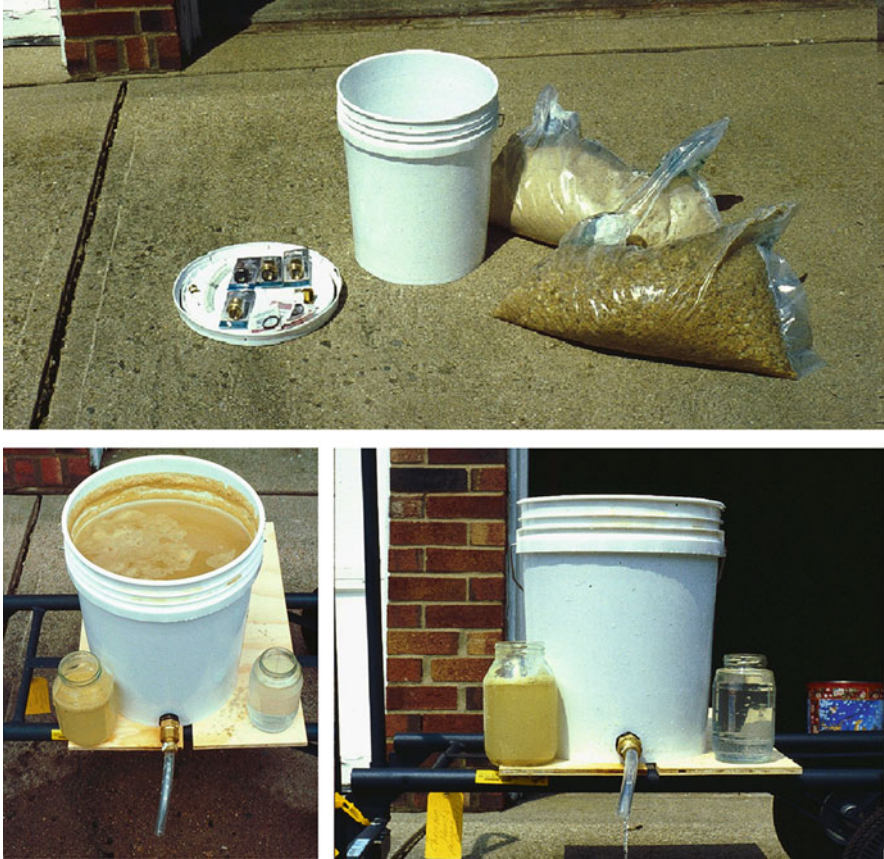
Fig. 8.15 This image shows a sand filter constructed from a 5 US gallon plastic bucket using some brass plumbing fittings, fine gravel and fine sand. The image on top shows the components used for creating the filter. The lower left image shows the filter with naturally turbid water on top of the sand, the glass jar on the left holds a sample of that naturally turbid water before filtration, and the glass jar on the right shows a sample of that same water after having passed through the sand filter. The lower right image shows a frontal view of the filter, plus the samples of naturally turbid water and filtered water. Use of these images is courtesy of the author
