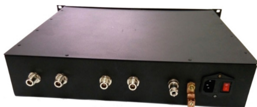
Fig. 8. Appearance of the modem device (right to the left: WTY0122 type connector with the button “Power 220 V”, DN 3 - control, N type - IF signal RX1, type N - IF signal TX1, N type - IF signal RX2, Type N - TX signal TX).
