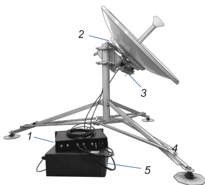
Fig. 6. Compact TRRS: 1 - modem device; 2 - antenna-rotating device; 3 - transceiver unit; 4 - cables; 5 - power supply.
