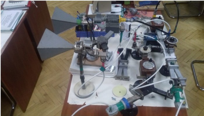
Fig. 13. Photo of the transmitting station of the proposed simplex RRCL
