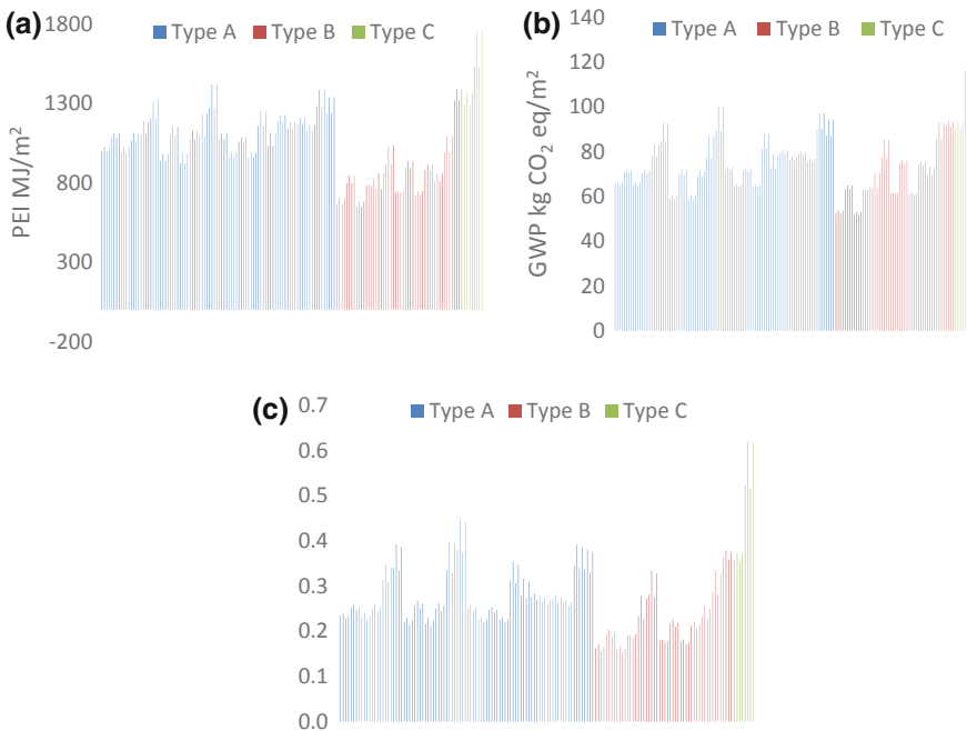
Fig. 1 Primary energy (a), Global warming potential (b), and Acidification potential (c) of the evaluated structures
