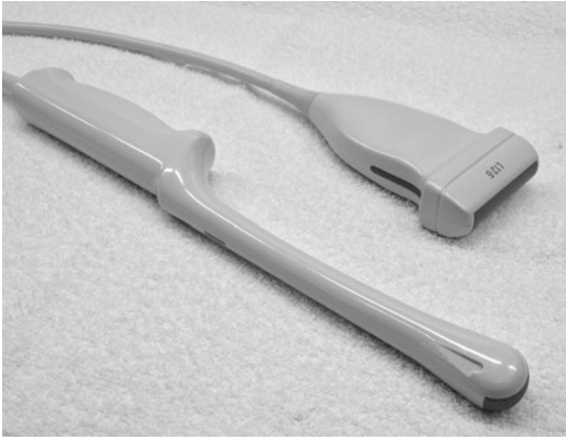
Fig. 13.1 Ultrasound probes: photo shows a high-frequency, linear array transducer above and a curved array endocavitary transducer below
