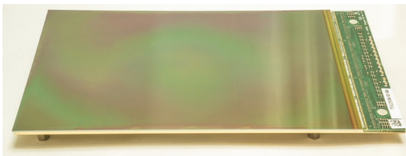
Fig. 2.14 A medium-sized CMOS image sensor, 150 \times 100 mm with 100 \mu\text{m} square pixel size. Note that it can be tiled, on three sides out of four, with other like sen-
