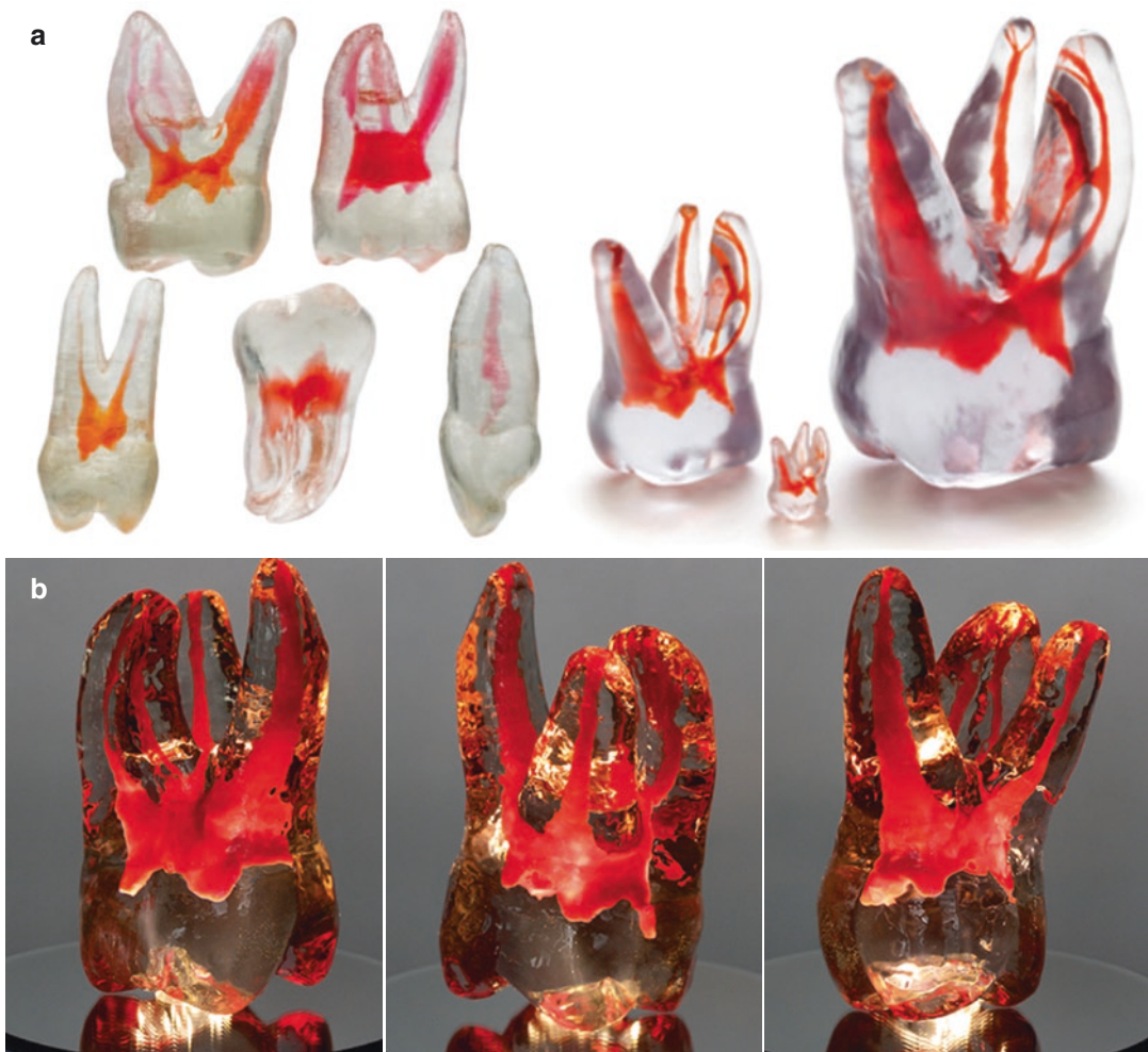
Fig. 12.19 Replicas of various teeth manufactured from corresponding real-tooth micro-CT scans using 3D printing technology in assorted sizes for didactic or teaching purposes. (a) True Tooth® (images available at https://den-
