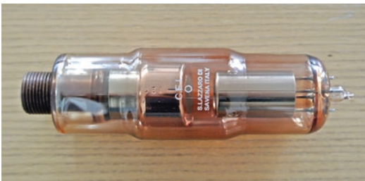
Fig. 2.3 An X-ray tube, stationary anode type
