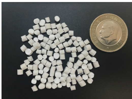
Fig. 19.2 Compound granules including 50% calcium carbonate and 50% LDPE produced in this study. The diameter of the coin is 26.15 mm
