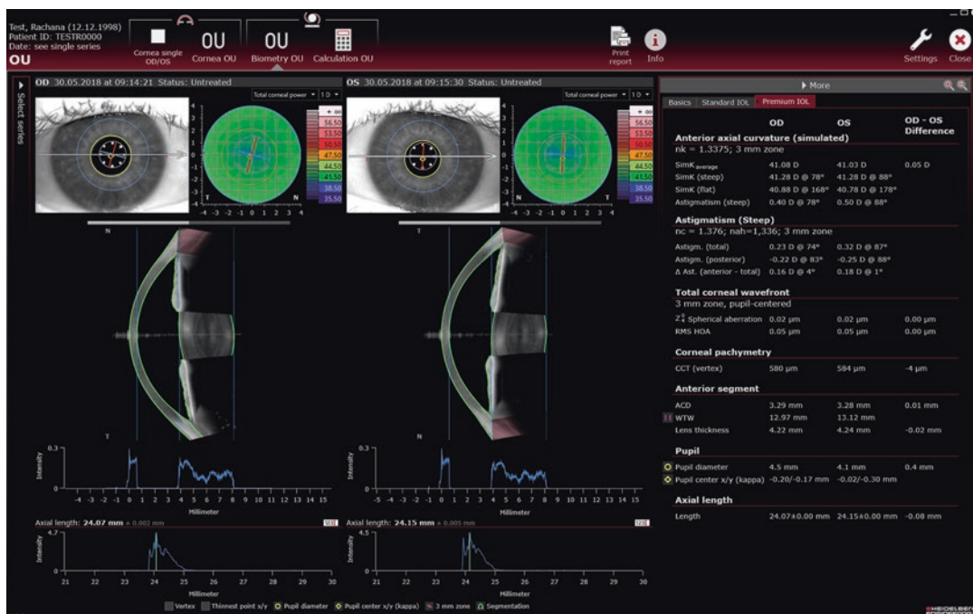
Fig. 13.12 ANTERION Cataract App both eyes (OU) view. Total corneal power maps, anterior segment OCT section image and OCT intensity graph, axial length diagram and anterior segment parameters of a patient with cataract
