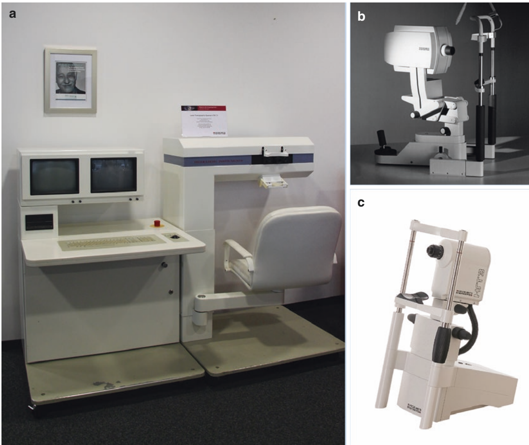
Fig. 2.5 Three generations of confocal SLOs for optic nerve head (ONH) tomography built in Heidelberg. (a) Laser tomographic scanner (LTS) from Heidelberg
