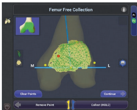
Fig. 11.5 Femoral surface is painted to build the virtual model using the optical probe
