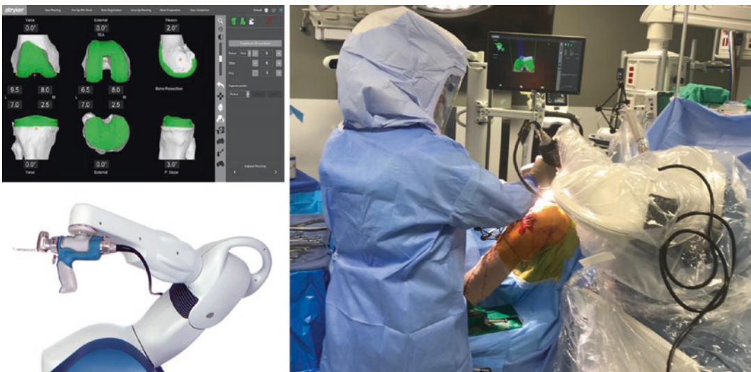
Fig. 2.4 MAKO planning, instrumentation, and intraoperative use for distal femur resection. (Operative photo courtesy of Steven Myerthall, MD, The CORE Institute; MAKO photo courtesy of Stryker, Kalamazoo, MI, USA)
