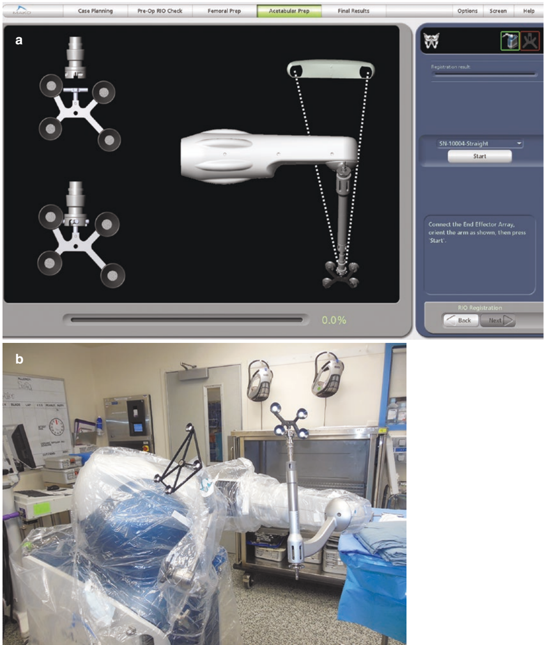
Fig. 20.4 (a, b) Before a surgical incision occurs, robot registration is performed by the end effector of the robotic arm, which is equipped with an array that has a series of reflective markers
