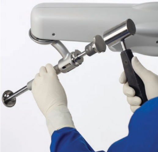
Fig. 20.9 Cup insertion occurs with line haptics, meaning the system will not allow deviation from the plane and the component orientation is “held” in the predetermined orientation. (Courtesy of Stryker, Kalamazoo, MI, USA)
