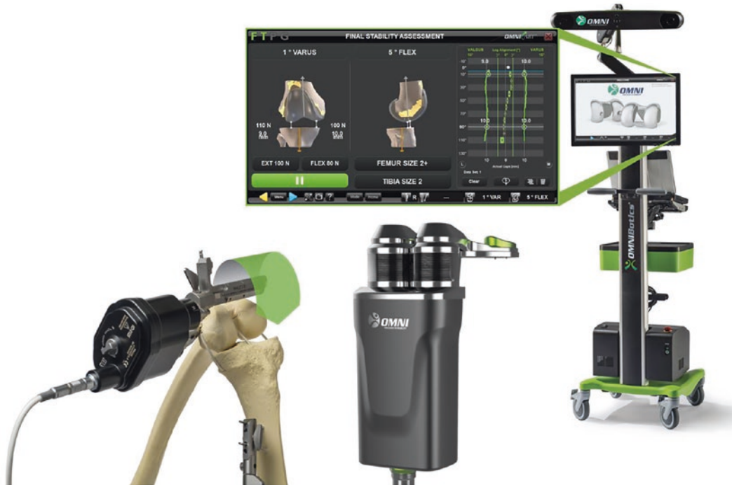
Fig. 17.1 The OMNIBotics® system – an image-free robotic-assisted TKA system that integrates intraoperative 3D anatomical modeling, real-time pre- and postoperative
