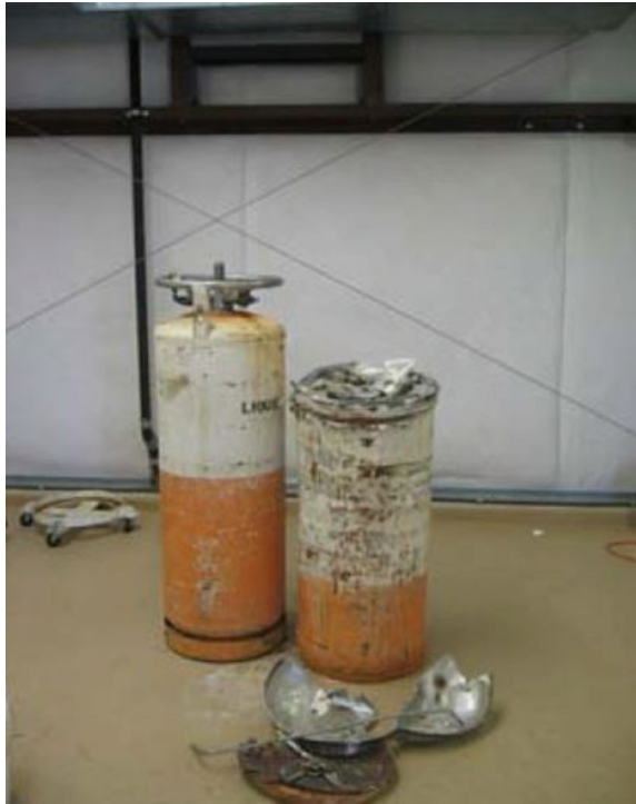
Fig. 3.3 The dewar which exploded on the right; a similar but undamaged dewar on the left
