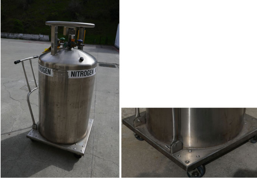
Fig. 2.2 LN 2 Dewar and transport cart. The close up shows the weld fixing the bottom of the Dewar to the cart. Courtesy SLAC National Accelerator Laboratory
