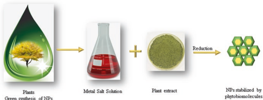
Fig. 1.6 Schematic representation of the mechanism of NP synthesis by plants
