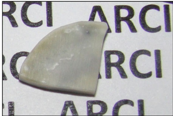
Fig. 16 Photograph of SPS sample processed with graphite foil after annealing
