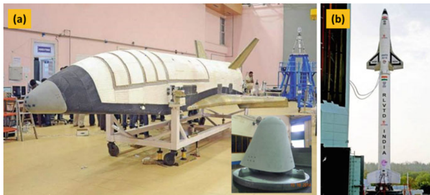
Fig. 40 (a) RLV-TD with SiC coated C/C composite nose cap (inset), (b) RLV-TD in launch pad [248, 250]
