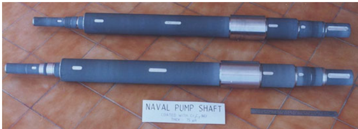
Fig. 16 Naval submarine pump shaft coated with wear and corrosion resistance \text{Cr}_3\text{C}_2 -25NiCr by detonation spray technique
