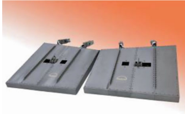
Fig. 18 X-38 Body flaps made of CVI and LPI-generated C_f/SiC Composites (with permission from publisher) [26]
