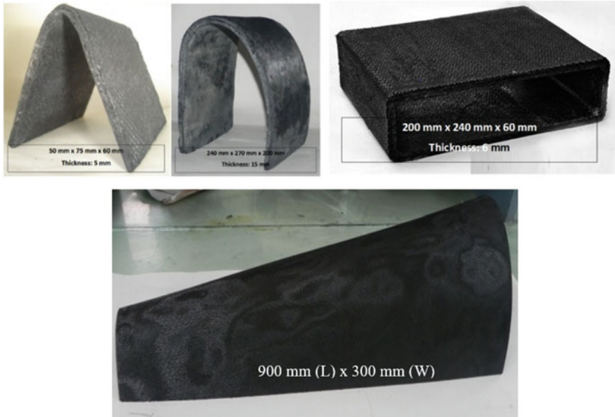
Fig. 31 Shaped CMC components from borosiloxane [209]
