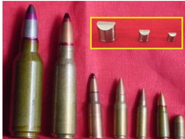
Fig. 26 Different caliber ammunition and fragment simulating projectiles
