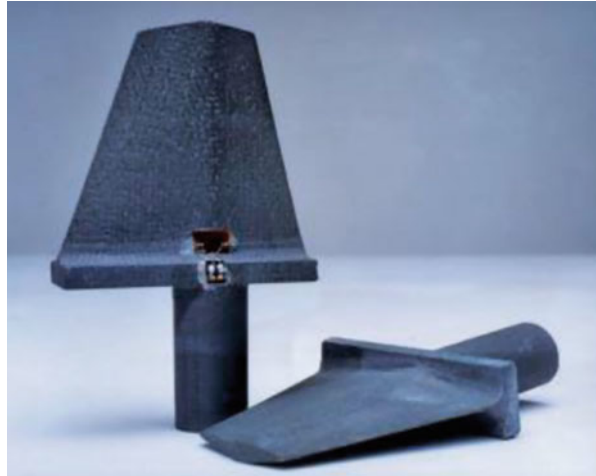
Fig. 20 LSI-generated C_f/C-SiC composites jet vanes developed by DLR (with permission from publisher) [26]
