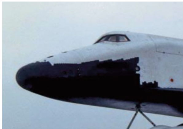
Fig. 17 LPI-generated C_f/SiC nose caps in Buran (with permission from publisher) [26]
