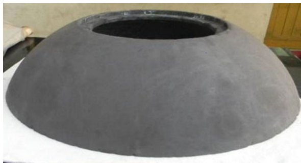
Fig. 46 SiC coated C/C noseshell (dia. 960 mm) with sealant coating [255]
