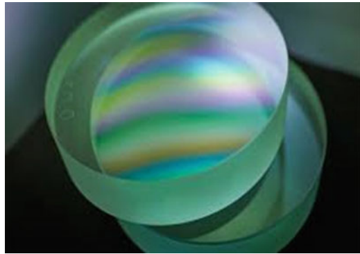
Fig. 20 Newton rings/Fringes formation at the contact of work piece and test plate
