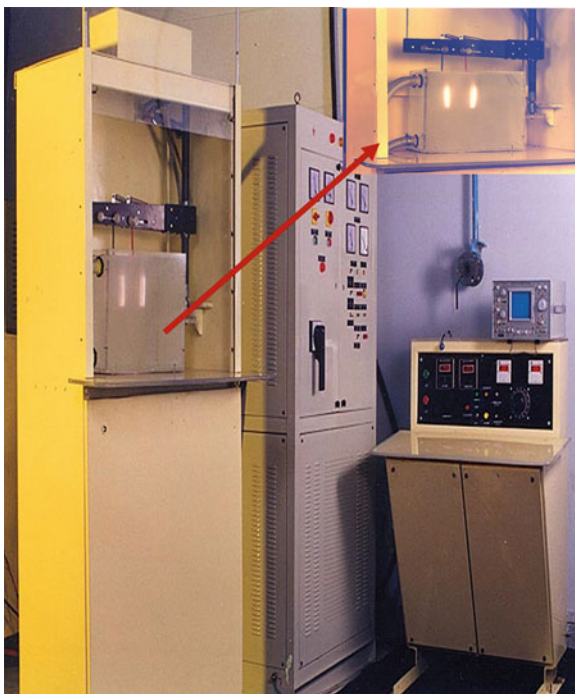
Fig. 19 Micro Arc Oxidation (MAO) lab scale equipment in operation illustrating control panel and reaction chamber (inset image) in which the component being treated exhibit illumination due to plasma discharges
