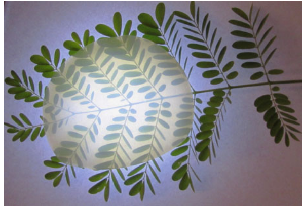
Fig. 2 Transparent silica aerogel made in the author's laboratory
