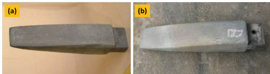
Fig. 43 SiC coated leading edge (width 15 mm; radius of curvature 1 mm): (a) before and (b) after exposure to arc-jet
