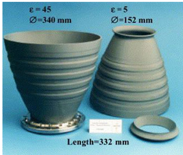
Fig. 23 (a) 150 N bipropellant C/SiC rocket engine, (b) hot fire of 150 N bipropellant C/SiC rocket engine. (Reproduced from Ref. [167] with permission from Elsevier)
