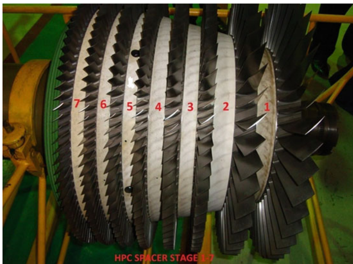
Fig. 10 Various turbine engine parts coated with \text{Al}_2\text{O}_3 coating
