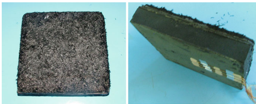
Fig. 64 Ceramic-ablative hybrid TPS after KHS test (two views)
