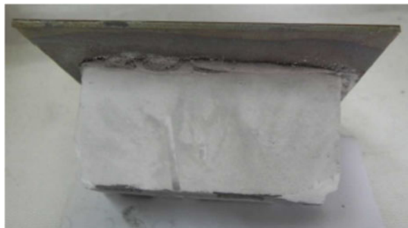
Fig. 56 Inconel/silica tile bonded specimen after heated to 500 °C in a muffle furnace [319]
