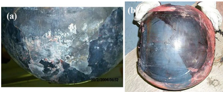
Fig. 13 Ball valve (a) coated with \text{Cr}_2\text{O}_3 and (b) coated with nano- \text{TiO}_2 after exposure to identical service life [67]
