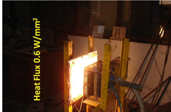
Fig. 26 Kinetic heating testing of C/SiC composites
