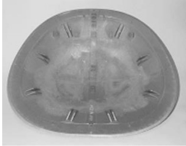
Fig. 21 Nose-cap of X-38 (NASA). (Reproduced from Ref. [165] with permission from John Wiley and Sons)
