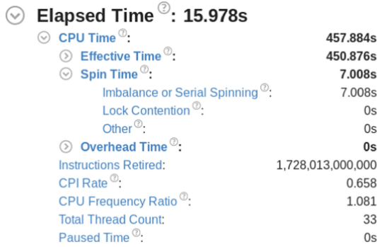
Fig. 4. Execution time obtained by an explicit work-sharing OpenMP-based TVD–Hopmoc method when studied with the support of the Intel ® Advisor shared memory threading assistance tool. Spin and overhead times add to the idle CPU usage value.
