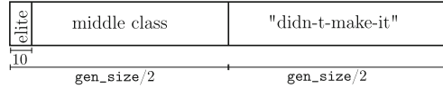
Fig. 2. Division of a generation’s population (size gen_size ) in classes that are then used as a factor for creating the following generation.
