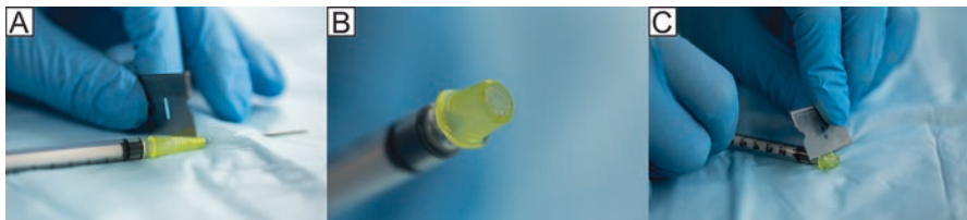
Fig. 6 Injury hub construction. Firmly attach a 20 gauge needle to a 1 cc syringe and insert the needle into a laboratory bench pad to prevent the needle from becoming projected after it is cut (a). Use a razor blade to cut off the tip of the needle (a). The injury hub is checked and refined for level (b). For the rat, the injury hub is beveled using a cosmetic pencil sharpener. Using a razor blade, score the exterior of the hub making burrs at even intervals around the hub (c). When finished, the cut end should be flat and even, and parallel to the Luer-Loc plane
