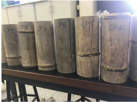
Fig. 2 Bamboo samples for compressive strength tests for Phyllostachys pubescens species. Source Author's own figure
