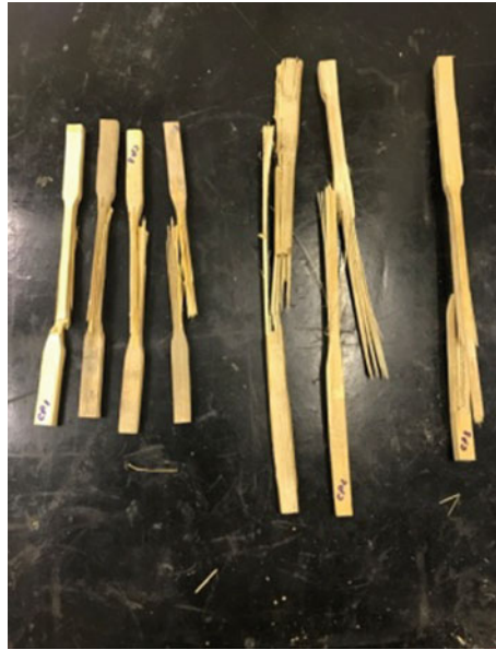
Fig. 11 Samples from both bamboo species: Dendrocalamus aesper and Phyllostachys pubescens . Source Author's own figure
