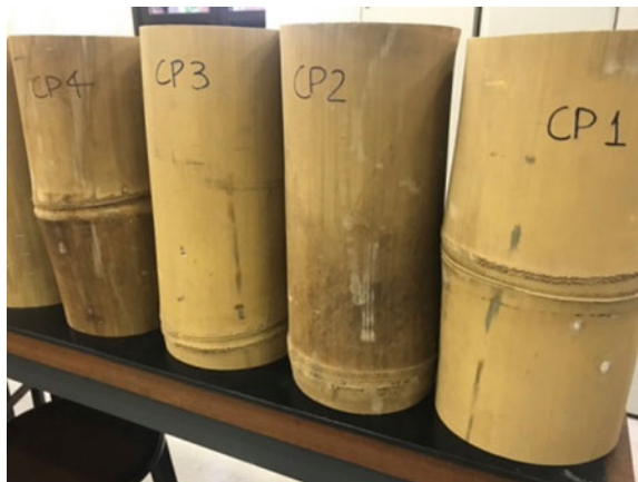
Fig. 1 Bamboo samples for compressive strength tests from the Dendrocalamus aesper species. Source Author's own figure
