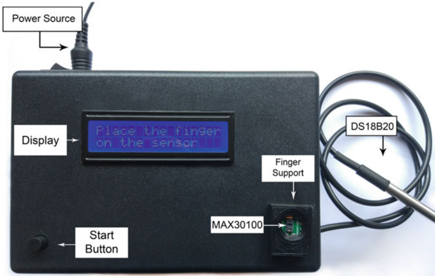
Fig. 5 Prototype of the monitoring system developed
