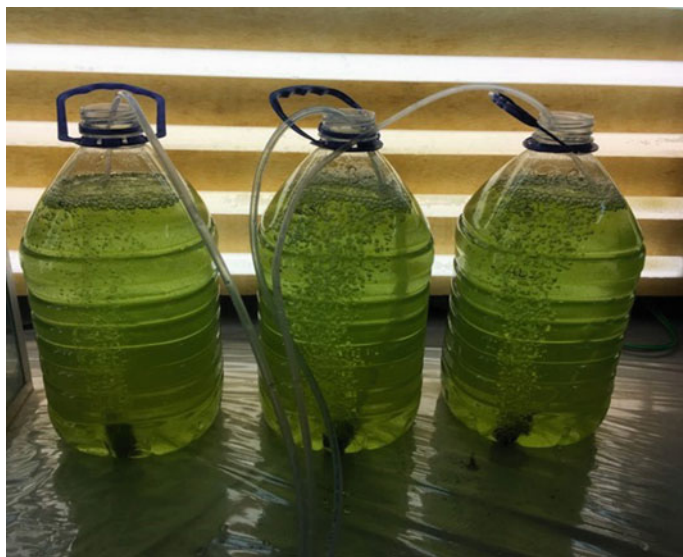
Fig. 1 Cultivation of Chlorella vulgaris in a medium containing effluent in batch photobioreactor
