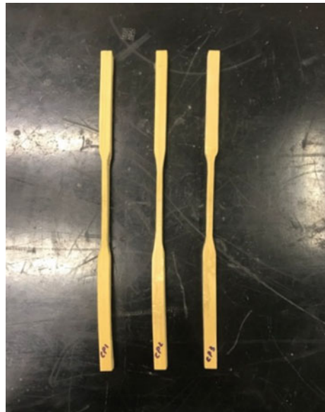
Fig. 6 Model for conducting the bamboo strip samples for tensile strength tests. Source Author's own figure
