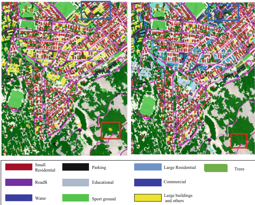
Fig. 3 On the left image all the large buildings were classified as single class. By the use of contextual information the single class was broken down into commercial and educational buildings
