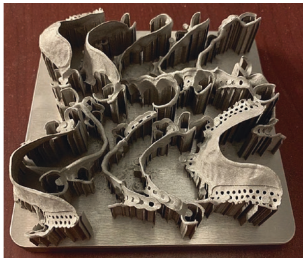
Fig. 5.12 A photograph showing the PRDP frameworks in the building platform processed by laser-sintering technology
