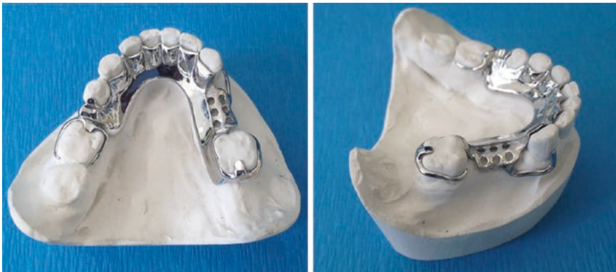
Fig. 4.12 Photographs showing the metallic framework of a partial removable dental prostheses (PRDPs) processed by the laser melting technology
