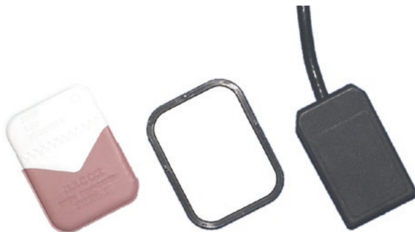
Fig. 2.4 An example of the different types of receptors in dental radiography. An E-speed film (left), a photostimulable plate (middle), and a charge-coupled device (right)
