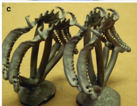
Fig. 5.14 3D printing for fabrication of partial removable dental prosthesis: (a) 3D-printed resin patterns of partial removable dental prostheses, (b) resin pattern of partial removable dental prosthesis framework with wax sprue ready for casting, and (c) metal frameworks of partial removable dental prosthesis cast from 3D-printed resin patterns
