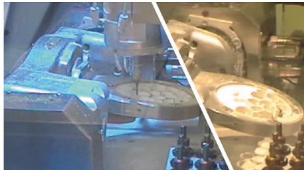
Fig. 4.5 Five-axis milling machine during drilling sequence
