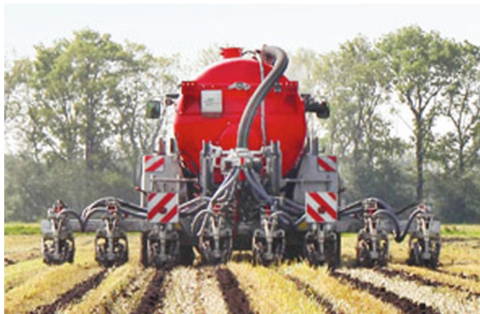
Fig. 27.10 Strip-till cultivator attached behind a liquid manure spreader. To prevent ammonium volatilisation, it is very important to avoid any delays of spreading manure (Edited by the author, courtesy of www.vogelsang.info )
