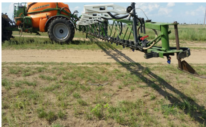
Fig. 37.6 Sprayer 'AmaSpot' 'Amazone' for weed control. Source Meinel (2014)
