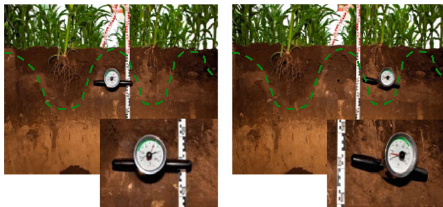
Fig. 27.8 Loosening of a Chernozem by strip-till near Bernburg in Central Germany (Grunwald 2012)
