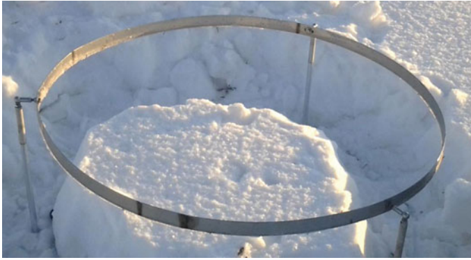
Fig. 12.3 Mechanical cutter to remove snow from the edge of the lysimeter vessel. Picture source Bondarovich, A. (January 2016)
