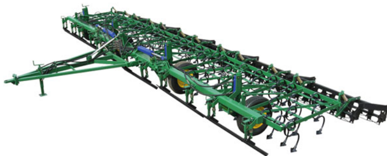
Fig. 27.16 KPSH9—Large-scale cultivator for medium depth tillage and seedbed preparation, three-rowed, heart or wing shares, here displayed with pusher blade, heart shares and tandem cage roller for a fine seedbed preparation ( http://agromehnika.ru/proizvodstvoKPSH.htm , 12.02.2017)
