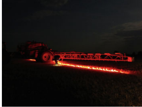
Fig. 28.7 Spot spraying technology on a conventional field sprayer—light sensors active for weed detection on the test farm PARTNER, Altai Krai 2014, during night work. Photo Grunwald (2014)
