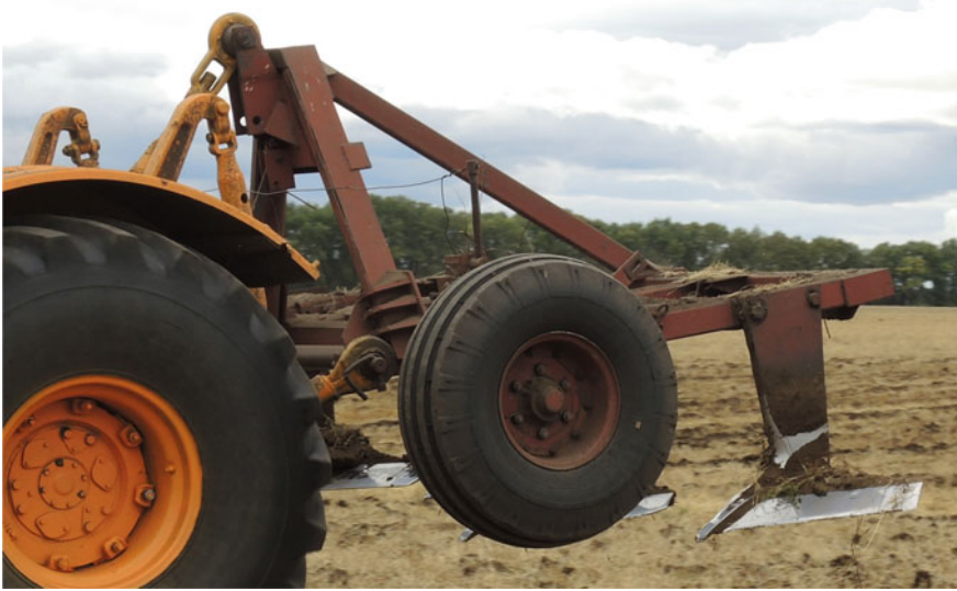
Fig. 27.17 PG 3-5—deep, large-scale cutting cultivator—mechanical erosion prevention and weed control ( photograph Grunwald 2013 )
