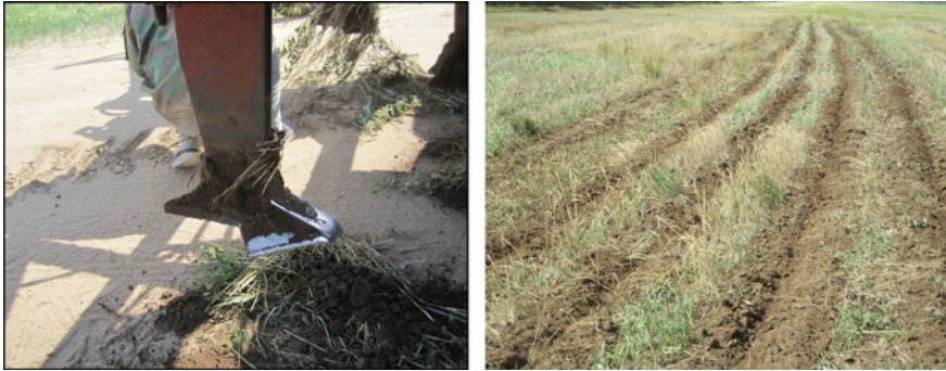
Fig. 27.12 Tine of a cultivator for large-scale deep tillage, now modified for strip-till after harvest (photographs Kozhanov 2011)
