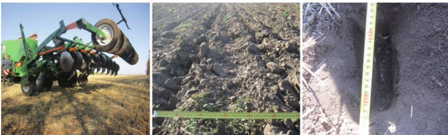
Fig. 27.13 First prototype of a strip-till cultivator by the Amazonenwerke—the tilled surface was still very rough because the cultivator was not equipped with tools to crumble the soil clods (photographs Kozhanov 2012)
