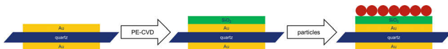
Fig. 3 Schematic of sample preparation procedure. After cleaning, the samples were coated with a thin SiO 2 film by means of PE-CVD. Subsequently, the sample was coated with SiO 2 particles with a diameter of about 250 nm (in analogy to [10])
