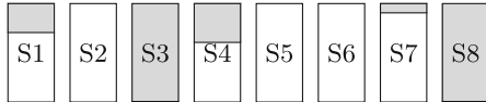
Fig. 1. An illustration of order-aware shard selection. Based on the predicted bucket ranking, portions of shards are selected (shaded area). While strongly relevant shards (S3, S8) may be fully processed, others could terminate early using GRC (S1, S4, S7), or be ignored entirely (S2, S5, S6).
