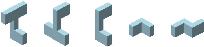
Fig. 9. Typical, pre-defined wiring and via patterns that have to be simulated by FEM in addition to those from Fig. 6.
