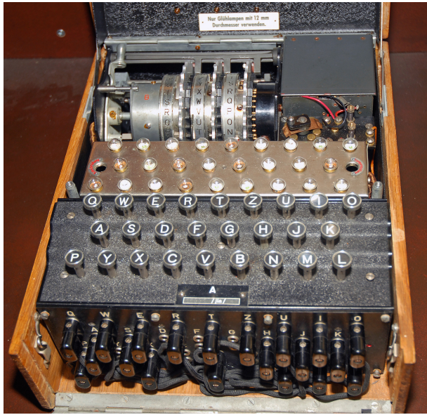
Fig. 1. Three wheel Enigma machine
