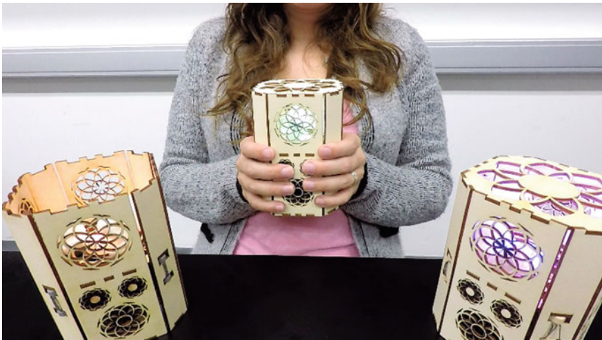
Fig. 6.2 Dišimo provides multimodal biofeedback about heart rate variability in order to encourage and help users focusing on their breath. Illustration courtesy of Jérémy Frey (Mladenović et al. 2018b)
