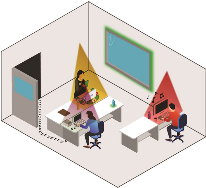
Fig. 6.8 Illustration of a playful ambient AR system to improve people’s well-being in the office. Projections can be used to highlight some elements (e.g. the window if the air quality is poor or a bottle of water if one person does not drink enough), to display footprints to suggest actions to users (e.g. taking a break), or to provide users with relaxing pictures (e.g. flowers on the desktop). Ambient lights can be used to help users focus on their work, or to indicate if someone is too noisy
