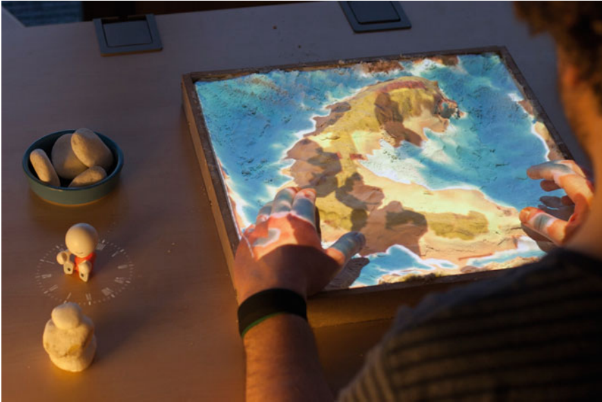
Fig. 6.7 The Inner Garden system is an augmented sandbox, the appearance of which changes according to the user's physiological signals. Inner Garden supports mindfulness practices (Roo et al. 2016). Illustration courtesy of Potioc project-team (Inria, Université Bordeaux, CNRS)
