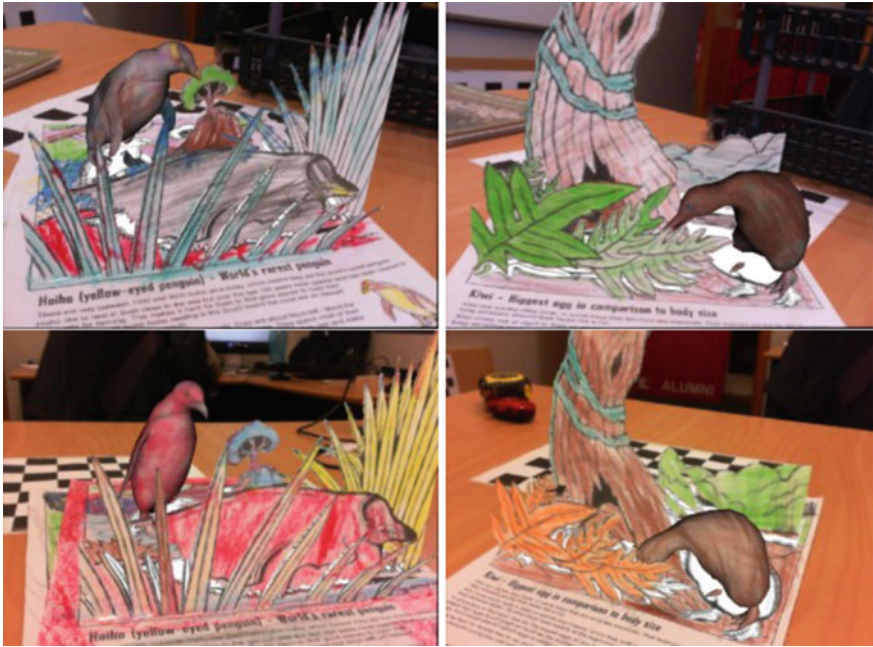
Fig. 3.10 Screen grabs of Augmented Reality Coloring Book (courtesy of HITLab NZ). Coloured 2D sketch is used for texturing 3D models
