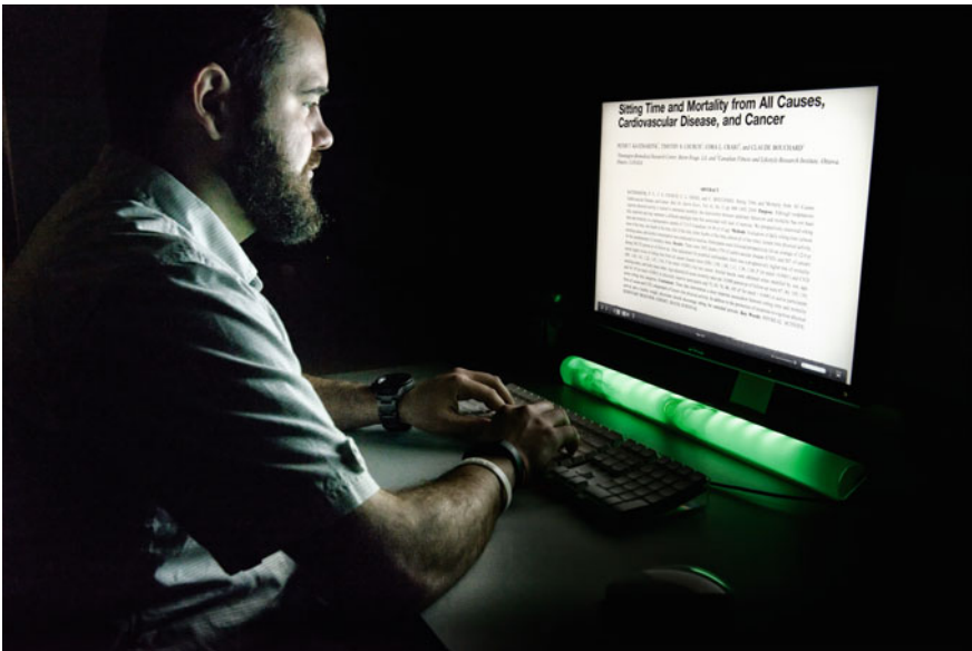
Fig. 6.3 The Health Bar prototype encourages users to take a break to reduce sedentary behavior (Mateevitsi et al. 2014). Illustration courtesy of Lance Long, Electronic Visualization Laboratory
