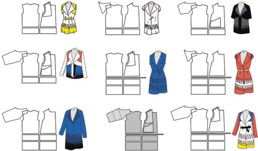
Fig. 3.9 Technical design of Tribute to Mondrian collection with related spare parts, shown in gray the ten-piece basic pattern
