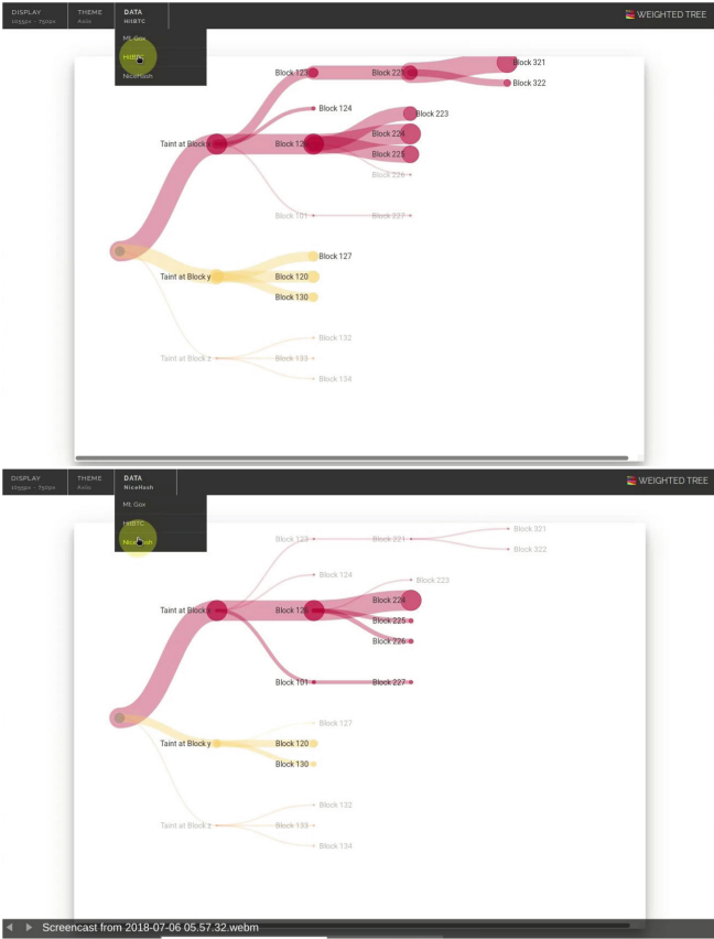
Fig. 8. These screenshots illustrate how the graph dynamically changes based on the taint type currently selected.
