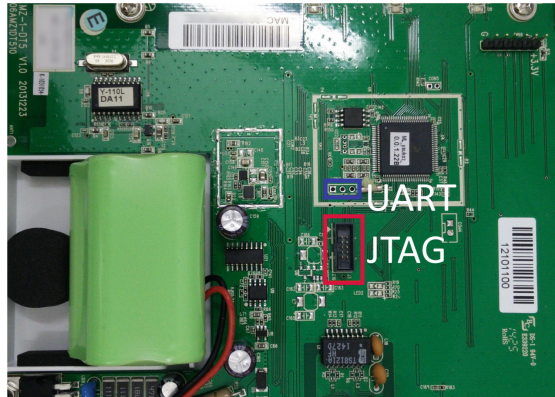
Fig. 2. Yale Easy Fit central unit PCB with UART and JTAG (Color figure online)
