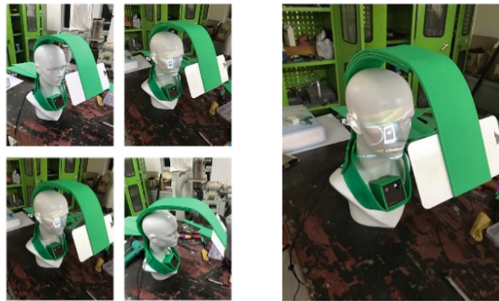
Fig. 19. Title: EVA fast prototype – Projection reflected to the mannequin face through a over the head mirror, 2018. (Source: Authors)
