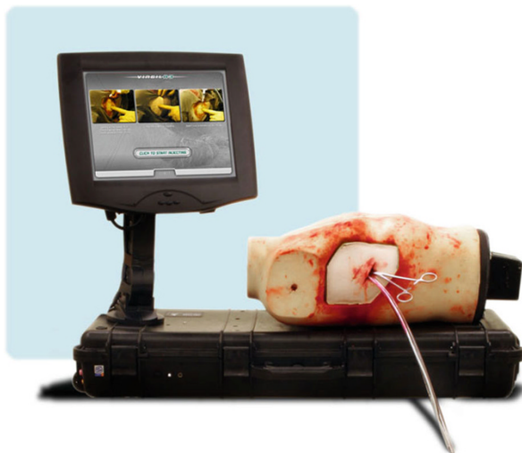
Fig. 1.5 The VIRGIL chest tube trainer developed in the Steve Dawson simulation laboratory at CIMIT/Massachusetts General Hospital. This demonstrates a part task trainer involving a PC-based graphical interface that tracks the internal position of chest tubes during training, providing a repeatable training experience superior to the use of live animals (Mark Bowyer, unpublished research results). Basic concepts of the VIRGIL system have been incorporated into the more comprehensive autonomous COMETS, now CAESAR, human manikin. Illustration courtesy of Dr. Steve Dawson
