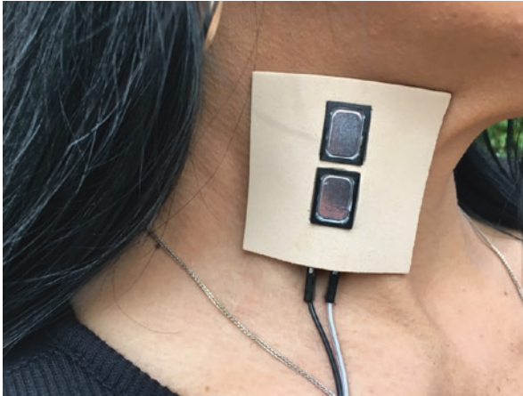
Fig. 20.4 A simulated pulse can be placed over a standardized patient's own pulse, in this case at the carotid artery. Associated circuitry provides a simulated pulse from 0–300 beats per minute, with either a regular or irregular rhythm
