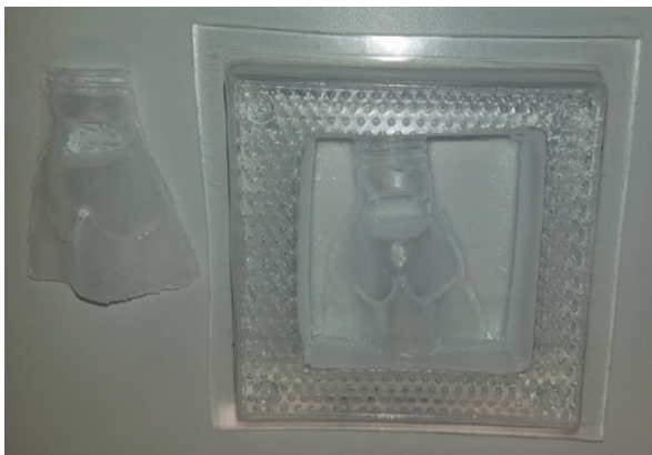
Fig. 19.6 Shows a thermal formed plastic mold of a thyroid cartilage for use with a cricothyroidotomy task trainer
