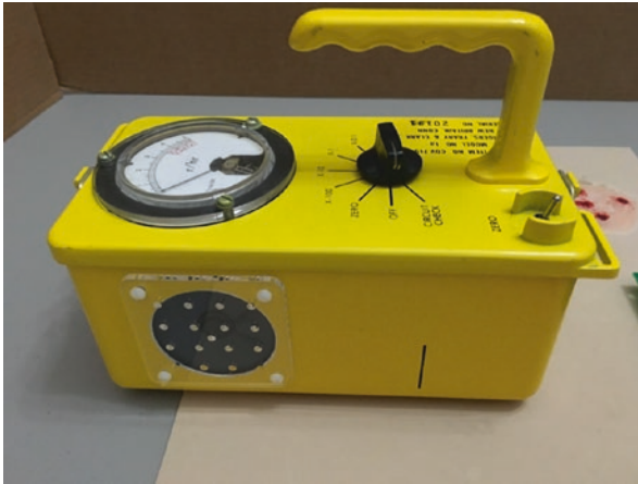
Fig. 20.2 This cold war Victoreen CDV-715 radiation survey meter has been converted to read RFID tags and then to simulate a predetermined amount of radiation with each tag. Similar RFID tags are used in corporate ID badges and can be read through a manikin skin or moulaged wounds. RFID tags also can be placed safely on a standardized patient (actor), since no actual ionizing radiation is present
