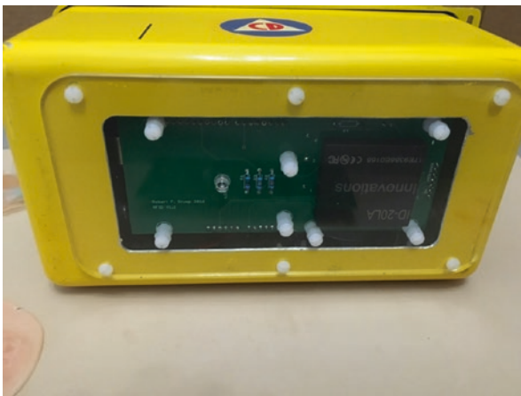
Fig. 20.3 The bottom of the simulated radiation detector, displaying the RFID reader, and associated home-brew circuitry
