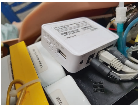
Fig. 14.8 Shows the selection switches on the router inside the SimMan3G Manikin. The switch options read Router, AP (Access Point), and Client. In Router mode, the box will create a network and assign IP addresses to any devices connected to the LAN port (right side of the box in the picture). In AP mode it will create an ad hoc wireless network with an SSID that can be searched for and used by the vital signs and control PCs. In Client mode, the router can be configured to allow connection to a larger network where IP addresses are assigned or reserved by a router outside of the manikin
