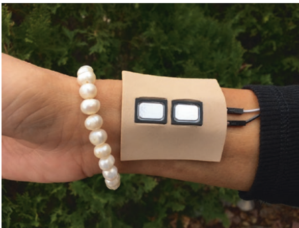
Fig. 20.5 A simulated pulse-generating speaker is placed over the standardized patient's radial pulse
