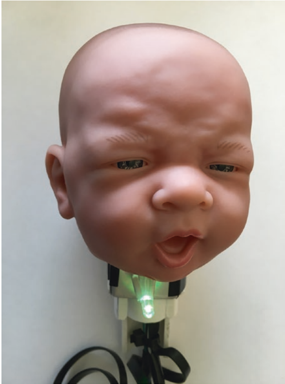
Fig. 20.7 Radio-controlled electronics assembly with LED is inserted into the doll's head
