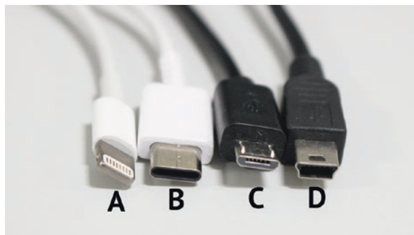
Fig. 11.23 A USB lightning cable (male); B USB-C cable (male); C USB-micro cable (male); D USB-mini cable (male)
