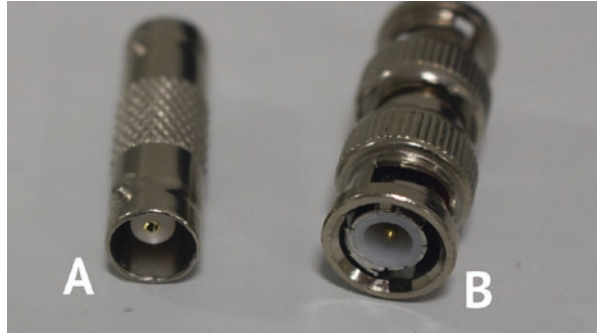
Fig. 11.18 A BNC female connector; B BNC male connector
