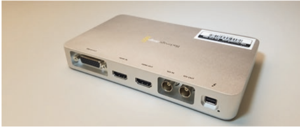
Fig. 19.2 Blackmagic Design UltraStudio Express media adapter. This type of box can convert High-Definition Multimedia Interface (HDMI) or Serial Digital Interface (SDI) signals into one of several digital formats for local display, recording, or internet broadcast
