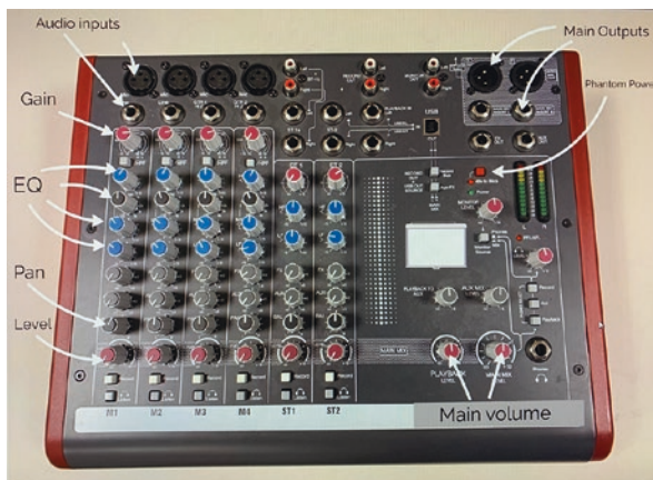
Fig. 11.7 The audio mixer is broken up into channels (M1-ST2) where inputs accept audio connections from XLR, Tip Ring Sleeve (TRS), and RCA-type connectors. The volume and tone of each channel can be sculpted and mixed with other audio channels. The final mono or stereo mix is sent to amplified speakers for the live main volume in the control room and simultaneously outputs another playback mix that is distributed by cabling to a recording medium like an audio encoder, digital video recorder (DVR), hard disk recording system, or digital audio server
