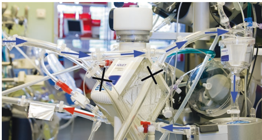
Fig. 15.1 Minimal invasive extracorporeal circulation system consisting of the main line. The system is characterized by a closed circuit, minimized dead space, biocompatible coating of the tubing system, and active air bubble removal. Photographs are made by the authors (Norman Koch, MediClin Heart Center Coswig, Germany)
