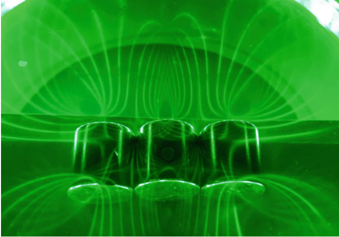
Fig. 1 Ferrocill using illumination of green LEDs with three magnets. The line pattern is formed due to the presence of magnetic field
