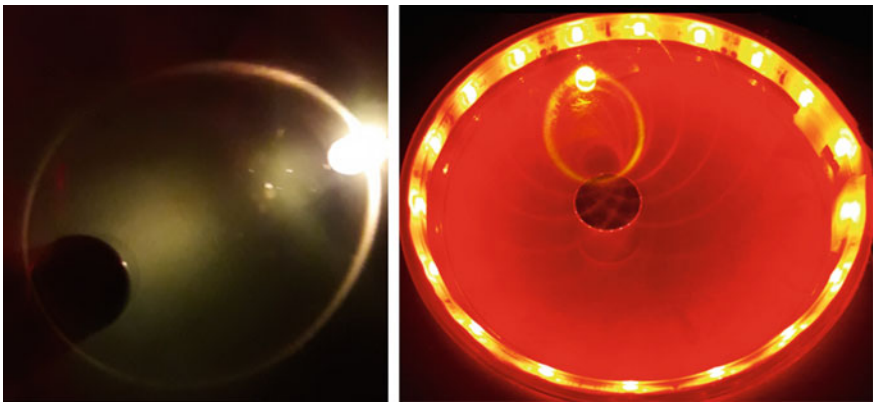
Fig. 6 The elliptical trajectory of light passing through the light source and around the face of a pole of the magnet is a limit cycle. We can see that each elliptical line is related to each LED
