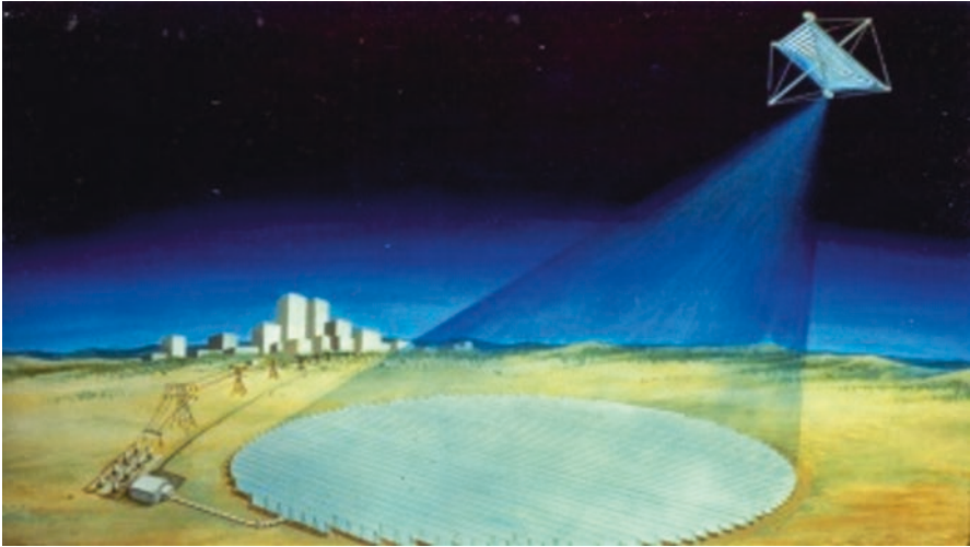
Fig. 8.4 Illustration showing a rectenna for SBSP reception plus an electrical power transmission system to an urban center.
