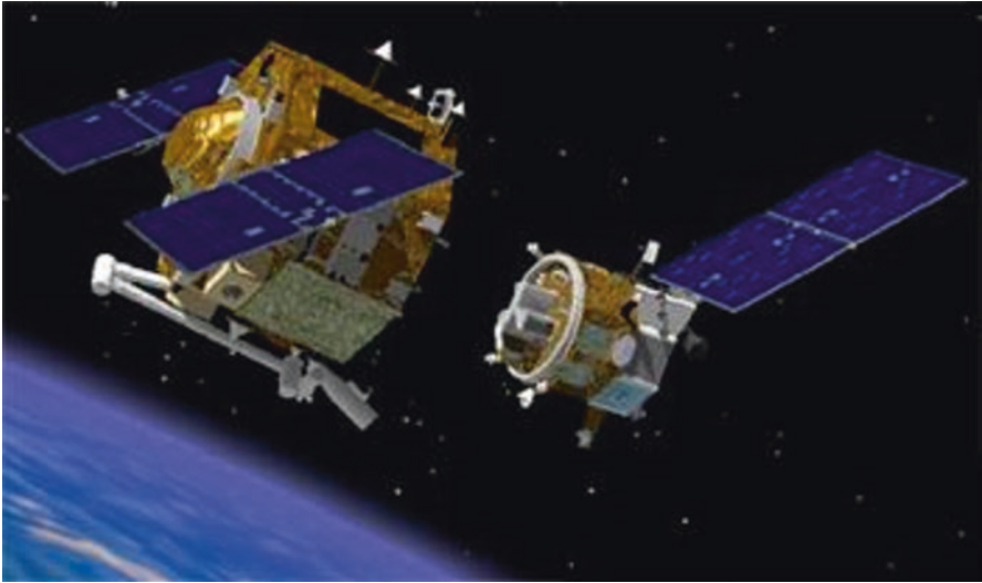
Fig. 7.2 Simulating the mating of the chaser Astro repair satellite about to capture the Next satellite. (Graphic courtesy of DARPA.)
