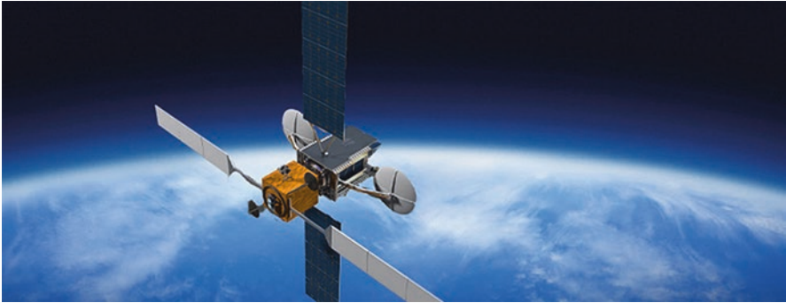
Fig. 7.6 The Vivasat MEV shown as mated with a satellite for servicing purposes. (Graphic courtesy of Vivasat.)
