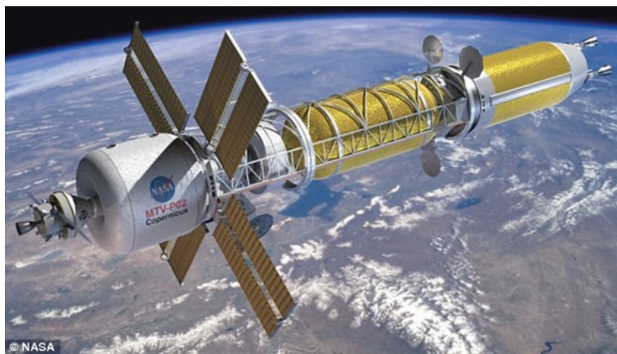
Fig. 11.2 Proposed nuclear thermal propulsion craft called Copernicus, envisioned by NASA to go to Mars. (Illustration courtesy of NASA.)
