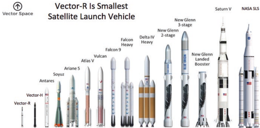
Fig. 10.4 The range in the size of launch vehicles keeps expanding. (Graphic courtesy of Vector Space.)
