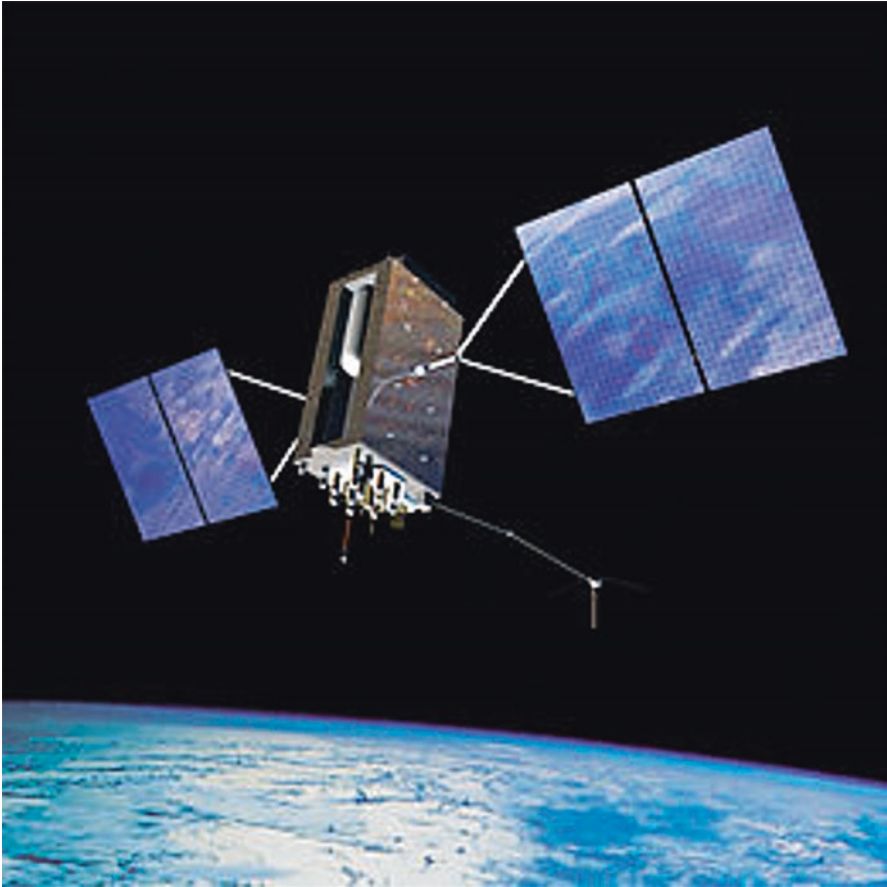
Fig. 4.3 The GPS Block IIIA Satellite Series. (Image courtesy of Lockheed Martin.)
