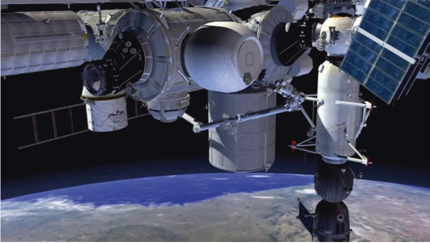
Fig. 12.4 BEAM Inflatable barrel-like structure as deployed on the Tranquility node of the ISS. (Graphic courtesy of NASA.)
