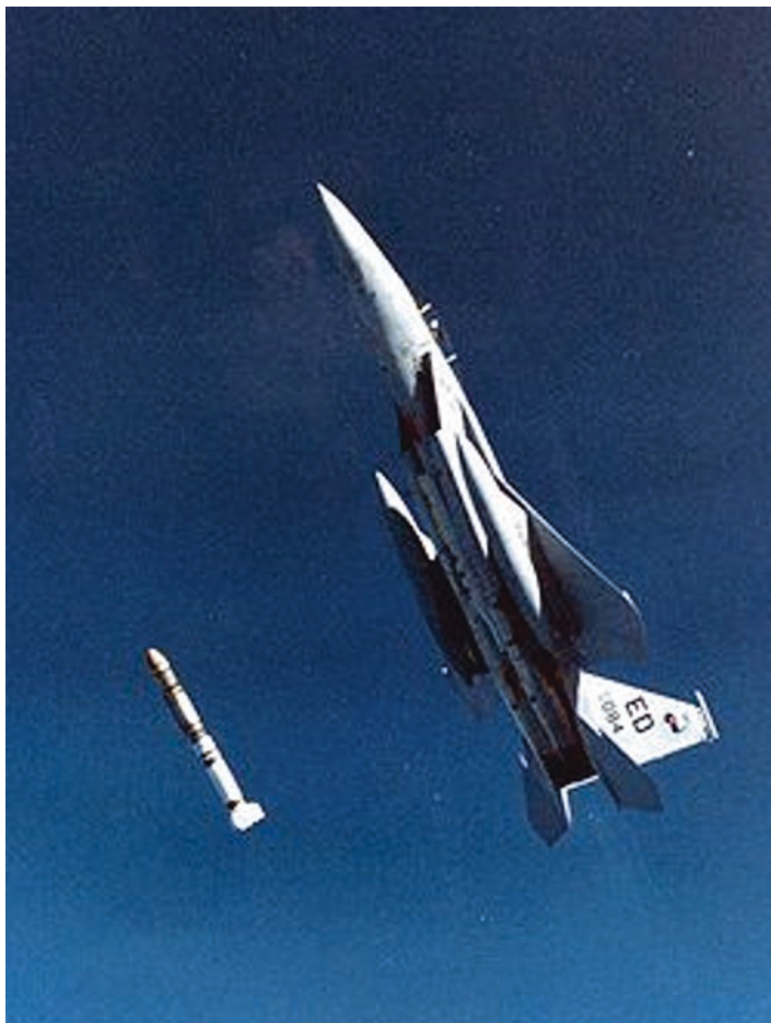
Fig. 9.1 U. S. Vought ASM-135 anti-satellite missile launch on Sep. 13, 1985, that destroyed its P78-1 target. (Graphic courtesy of the Global Commons.)
