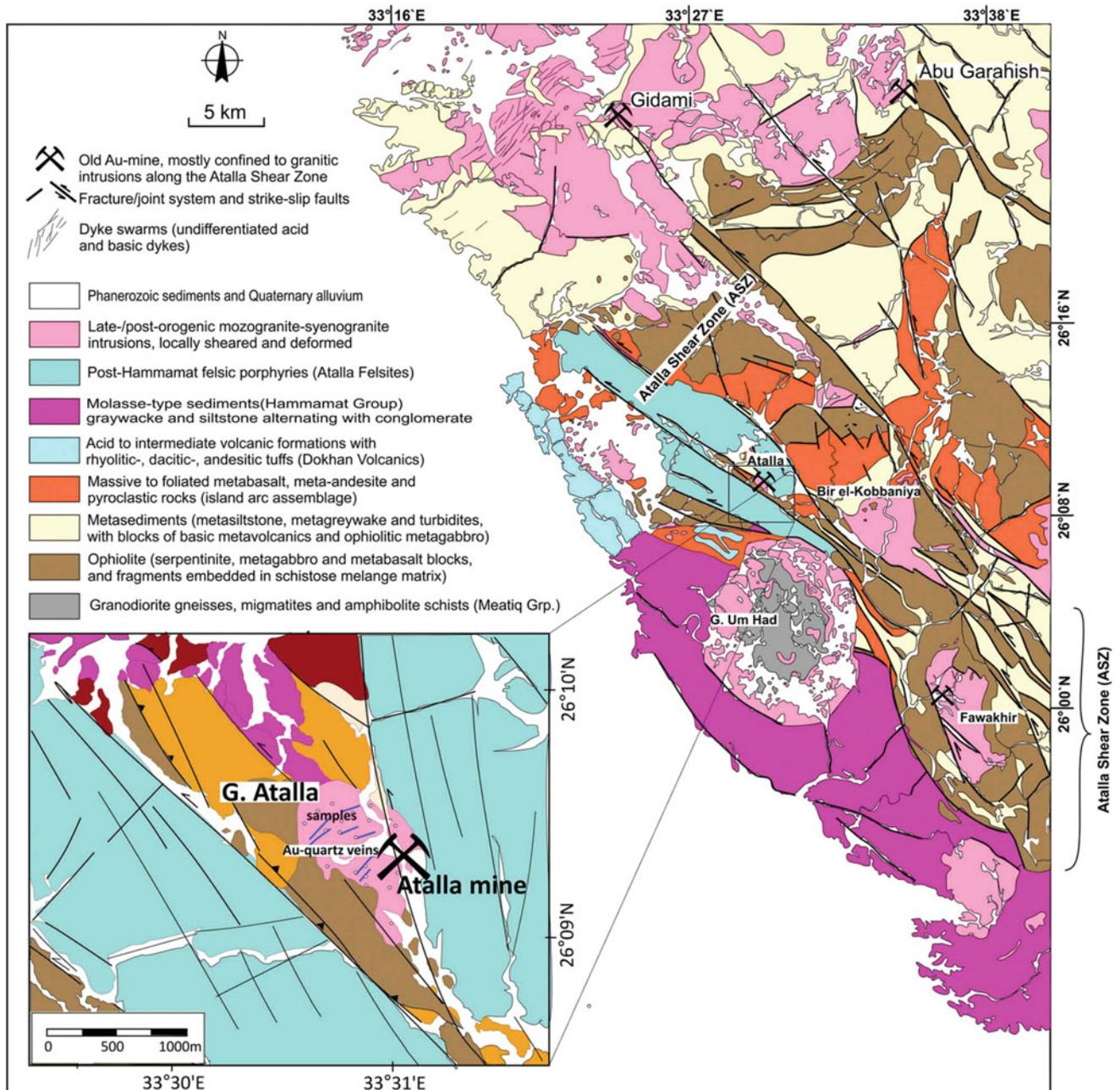
**Fig. 5.15** Geological setting of the Atalla shear zone (ASZ) and associated granitic intrusions and gold mineralization (Zoheir et al. 2018)
