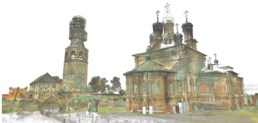
Fig. 4 3D point cloud of the Stroganov Complex of Usolye, derived from the laser-scanner survey. The figure shows the Transfiguration Church, the Bell tower and the Stroganov Chamber in the background
