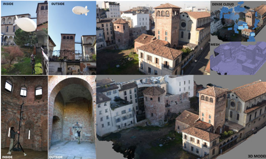
Fig. 4 Aerial and terrestrial photogrammetry to document the site and realise the 3D model
