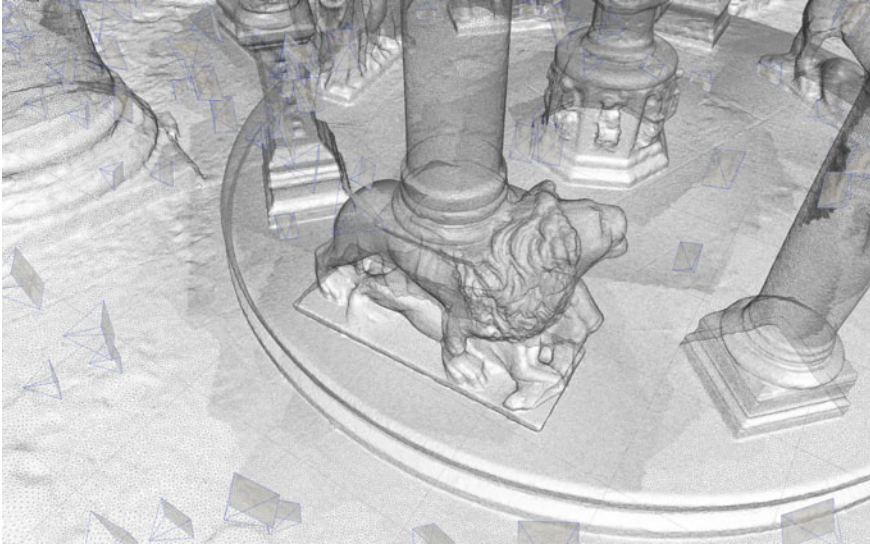
Fig. 13 Detail of the 3D mesh model where it is possible to see the resolution and the isometric triangles
