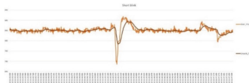
Fig. 3. Raw TP 10 values and the smooth TP 10 values of a short blink
