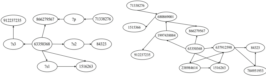
Fig. 3. A sample encoded query graph and RDF dataset over given RDF dataset.
