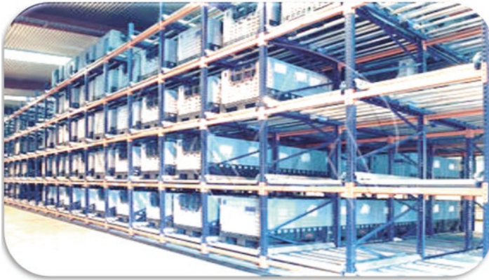
Fig. 4.8 Pallet live storage
