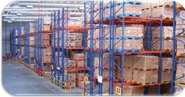
Fig. 4.6 Double deep racking
