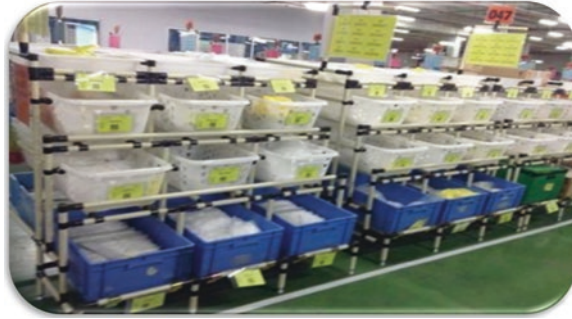
Fig. 4.10 Small parts live storage
