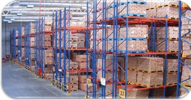
Fig. 4.6 Double deep racking
