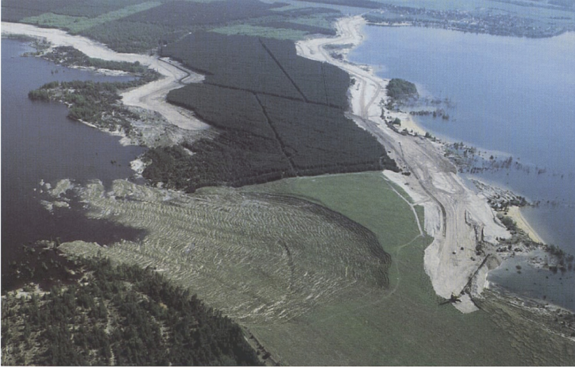
Fig. 6. Loose partly flooded sand deposit from lignite mining after flow slides (courtesy LMBV)
