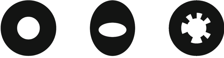
Fig. 2. Original (left), COS \Phi (middle) and WhyCode (right) localisation tags.
