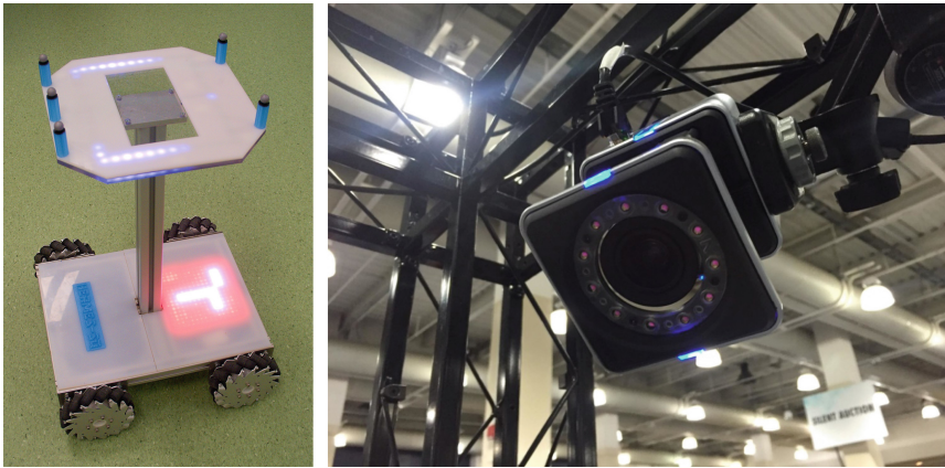
Fig. 6. Hermes SQ (left), Vicon localization system (right)
