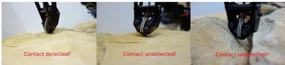
Fig. 3. Successful and failed detections with the version 1 of the foot force sensor
