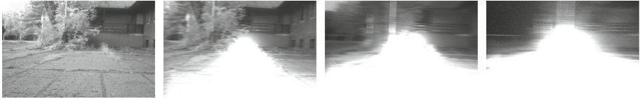
Fig. 14. Image blur caused by deteriorating lighting during a sharp turn. The left image was captured during the day, while the other ones were captured after sunset.
