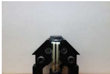
Fig. 2. Version 1 of the foot force sensor
