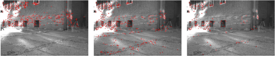
Fig. 8. The different setting of the keypoints detection: in the first image, 500 features are detected only from the top half. In the second image, the same amount is extracted from the whole image, and the last image has a fixed Hessian threshold, which results in feature deficiency.
