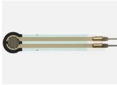
Fig. 1. Force-sensing resistor, courtesy of Interlink Electronics
