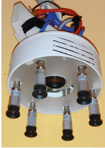
Fig. 3. Configuration of the gripper head with centered camera, suction cups and circular light.
