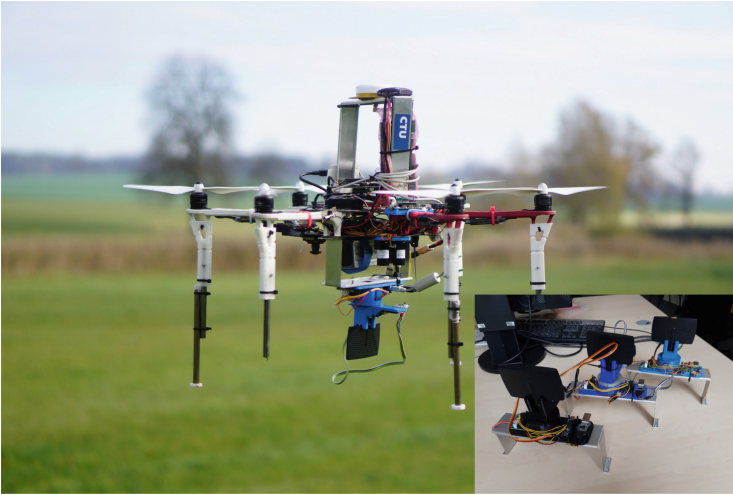
Fig. 1. MAV with directional antennas
