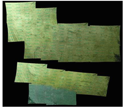
Fig. 11. Result of the Autopano stitching software applied to photos collected during mapping using the Wavefront algorithm.
