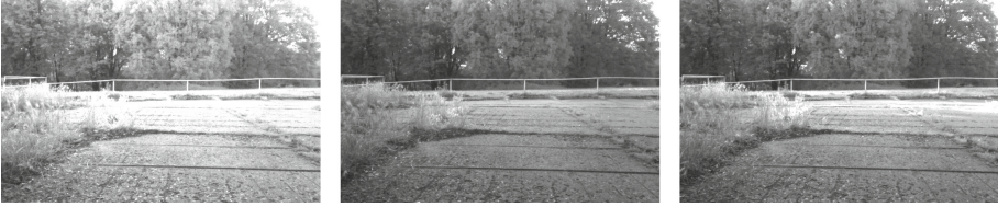
Fig. 6. Different exposure settings: the first image is captured with fixed exposure, the second with exposure control applied to the complete image and the last image was captured with exposure controlled according to the top half part of the images.
