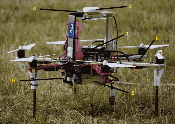
Fig. 1. MAV used in real platform experiments equipped with an essential list of components. (1) computer running ROS, (2) battery, (3) differential GPS - used for ground truth, (4) standard GPS, (5) a backup rangefinder not used in the presented experiments (6) Garmin rangefinder [17].
