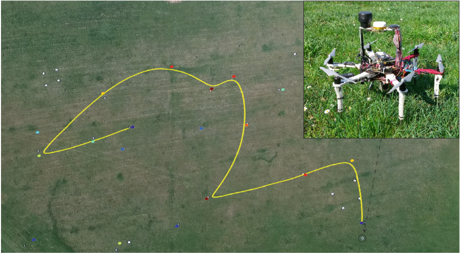
Fig. 1. An example trajectory used for information gathering task using hexarotor UAV found by proposed solution algorithm
