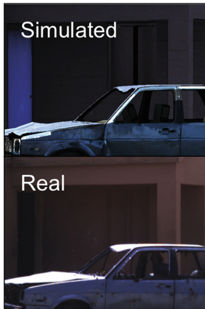
Fig. 2. An output image from a Sony CCD camera compared with the real object being modeled within the geo-environment.
