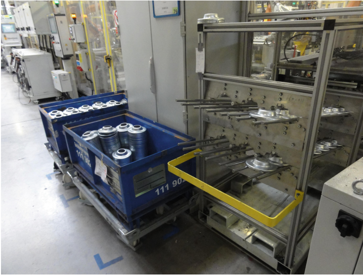
Fig. 1. Image of the transportation package with objects and feeder of the automatic assembly line
