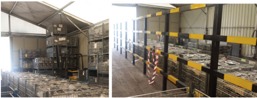
Fig. 5 Evolution of the area before and after the implementation of 5S—Security barriers
