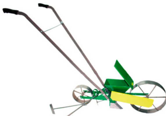
Fig. 8 SOR 1/1 vegetable single-row seeder with a brush-type sowing unit BBA 96/6, general view
