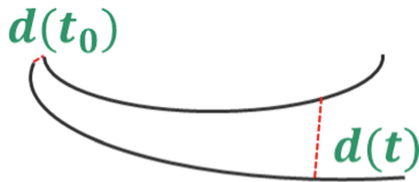
Fig. 1. A divergence of initially (i.e. at time instant t_0 ) nearby trajectories in the phase space.
